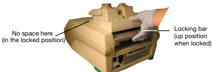
Figure 7. Locking the reaction module in place.
