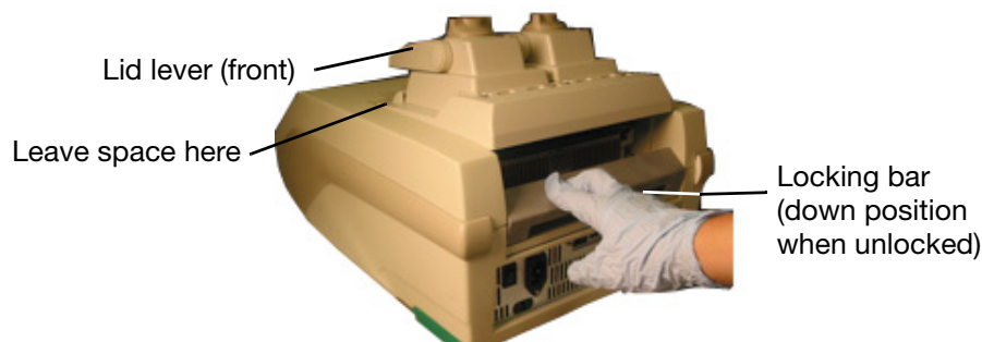
Figure 6. Inserting the reaction module into the bay.
