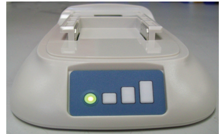
Receiving adequate power
