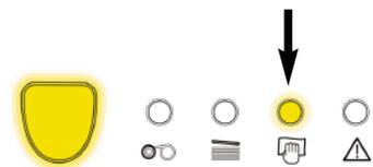
This message is an alert that indicates to the operator that it is necessary to perform the cleaning cycle. If the printer is not cleaned after the LED illuminates, the LED will remain illuminated and will start flashing when 200 additional cards have been printed.
