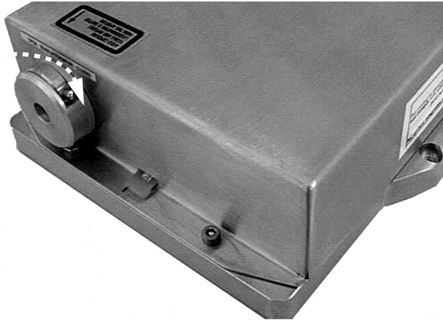
*Figure 5-1. Beam Shutter Closed*
