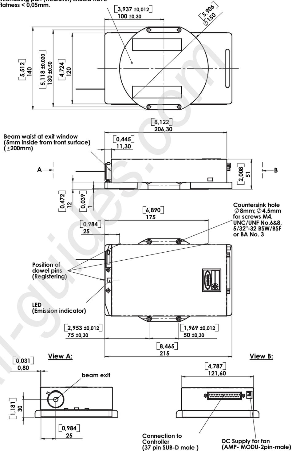
Figure 2-4. Sapphire Laser Head Dimensions
