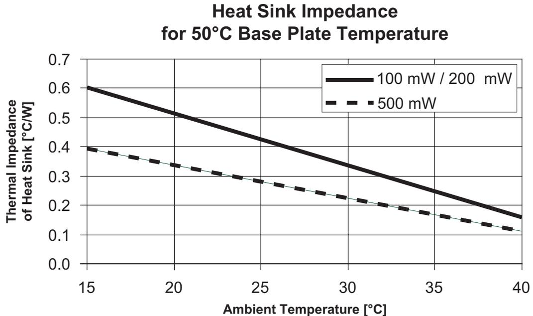
**Figure 3-2. Heat Sink Requirements**
