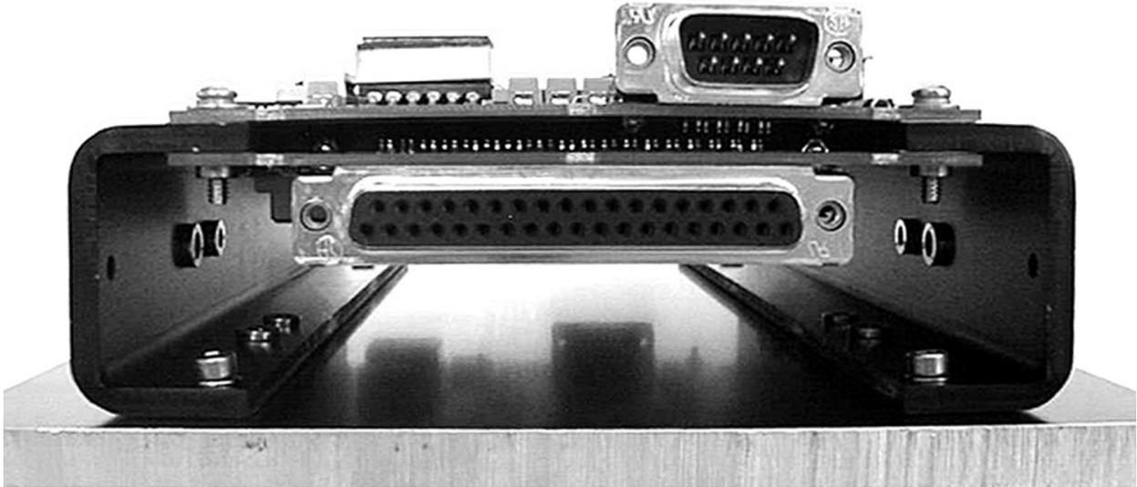
*Figure 3-4. Mounting of the Sapphire Controller*
