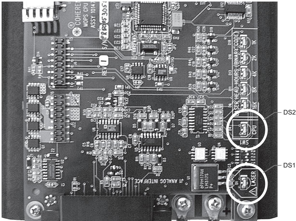
**Figure 4-3. LED Indicators on the Controller**
