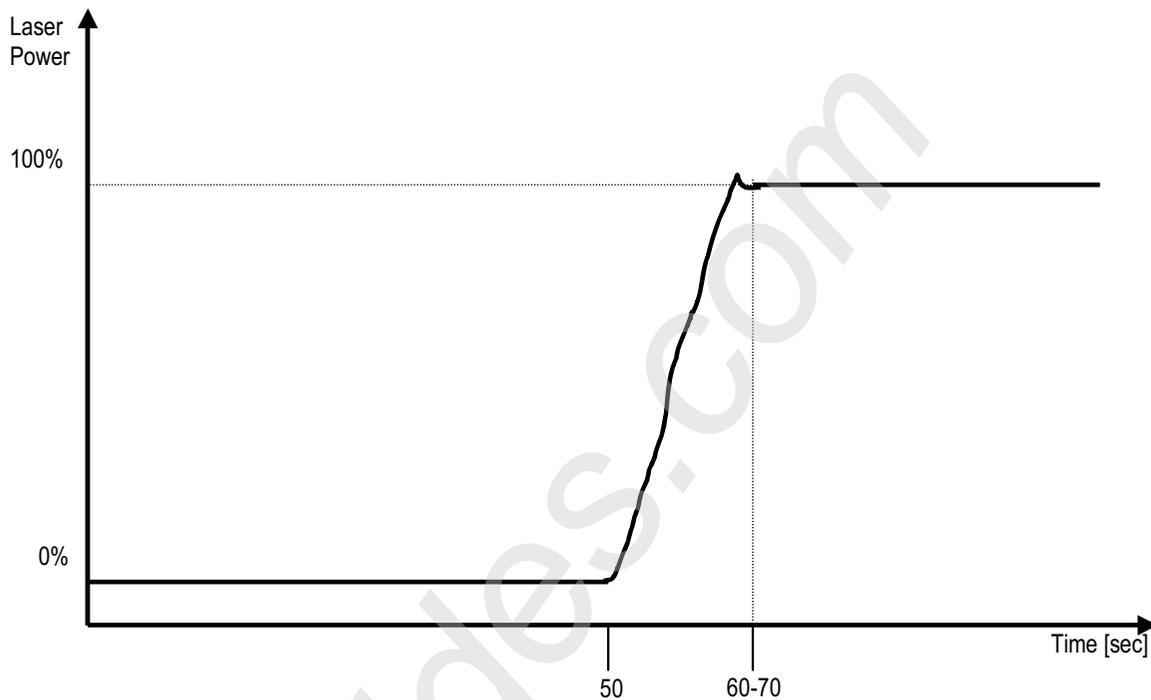
Figure 3-10. Typical Turn On Characteristics Diagram (from cold start)
