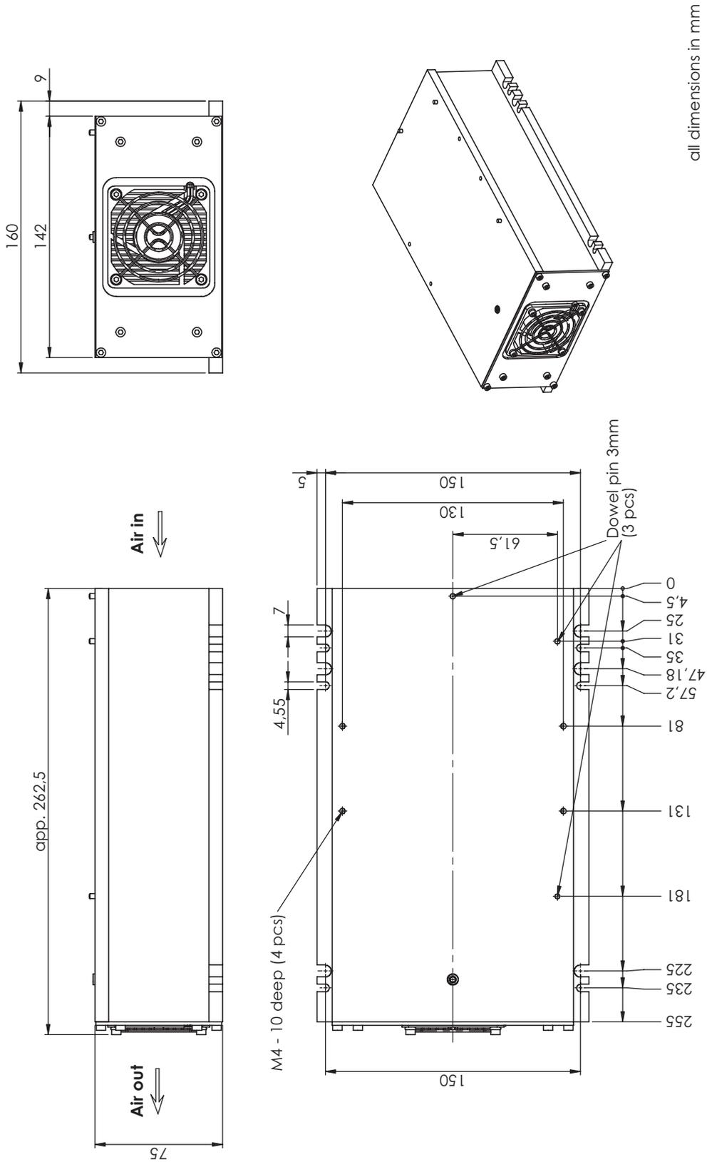
Figure 2-7. Optional Heat Sink for Laser Head Dimensions
