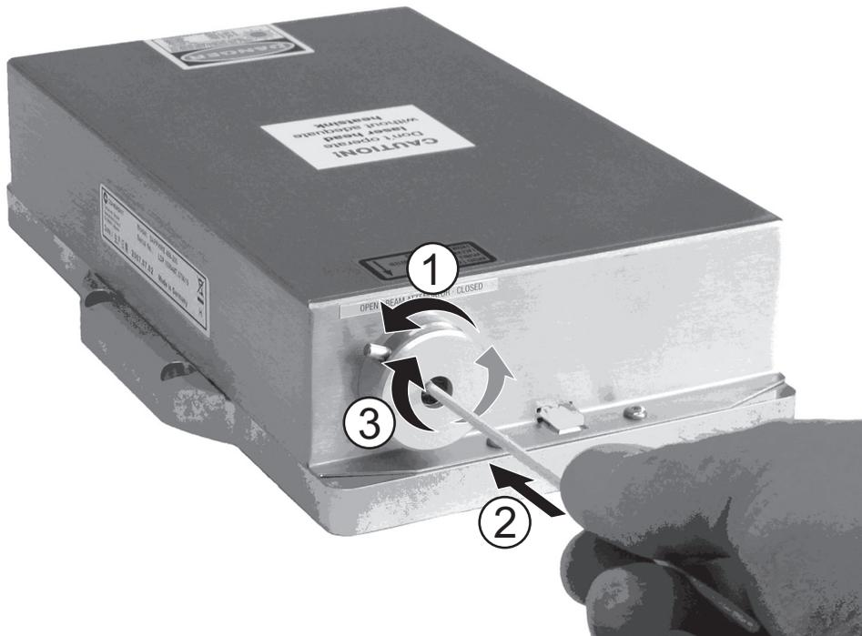
*Figure 4-2. Cleaning the Output Window*
