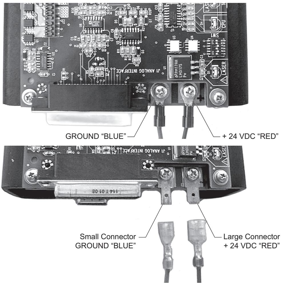
**Figure 3-8. Connecting DC Supply to Controller**
