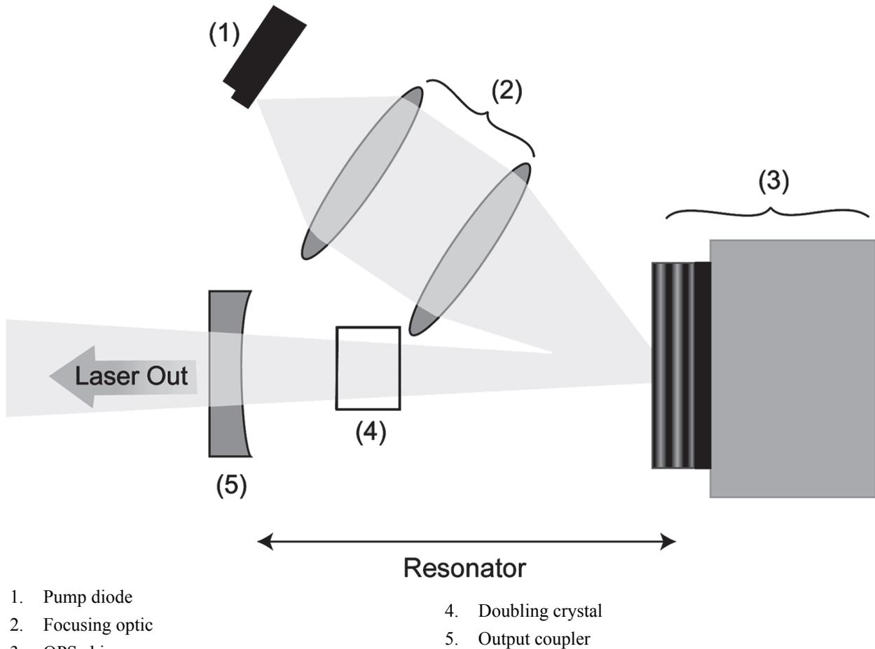
**Figure 2-2. Optical Schematic**
