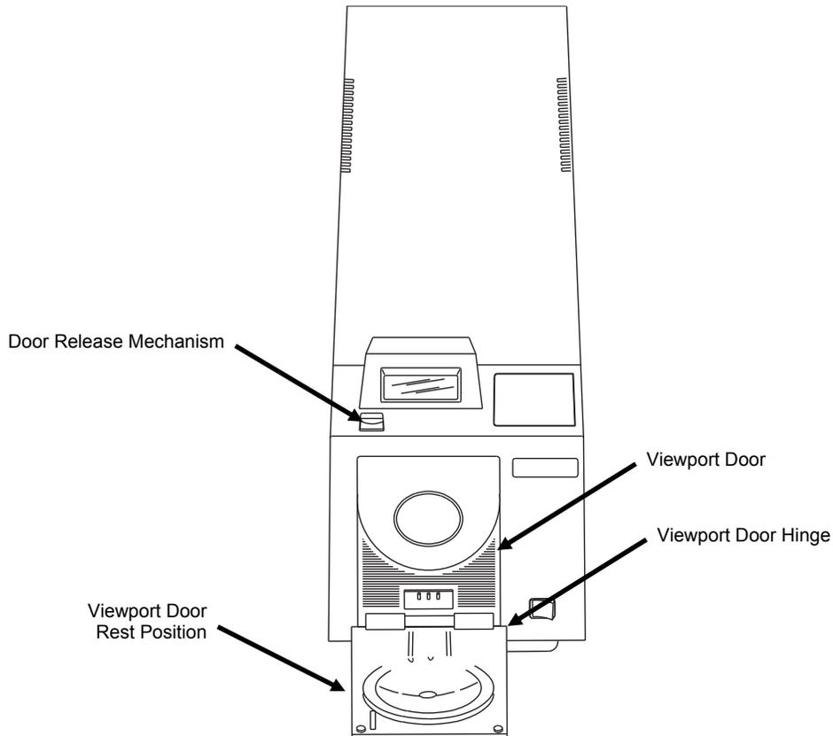
**Figure 4-3. Viewport Door Release Mechanism, Resting Position**
