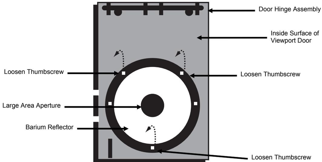
**Figure 4-7. Changing the Sampling Aperture, Step 2.**
