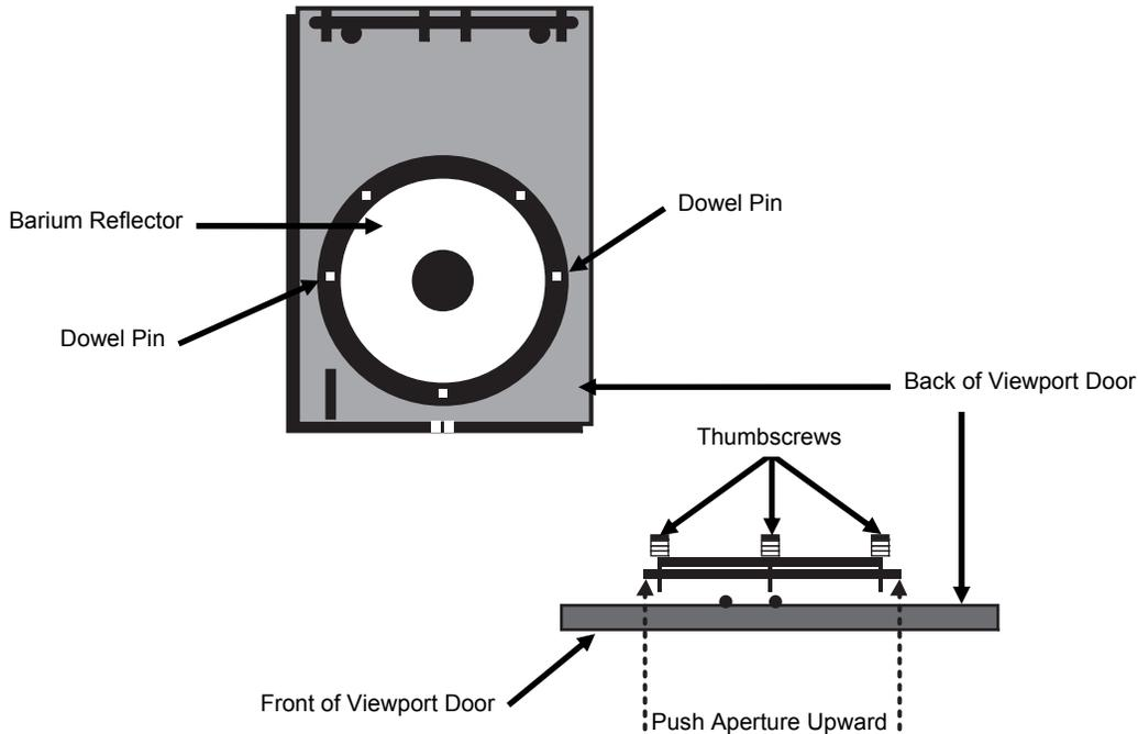
**Figure 4-8. Changing the Sampling Aperture, Step 3.**
