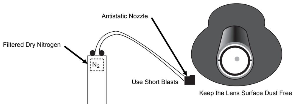
**Figure 5-3. Cleaning the Area of View Zoom Lens**
