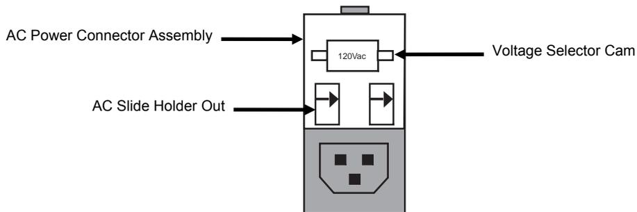
**Figure 5-8. Fuse Replacement, Step 5**
