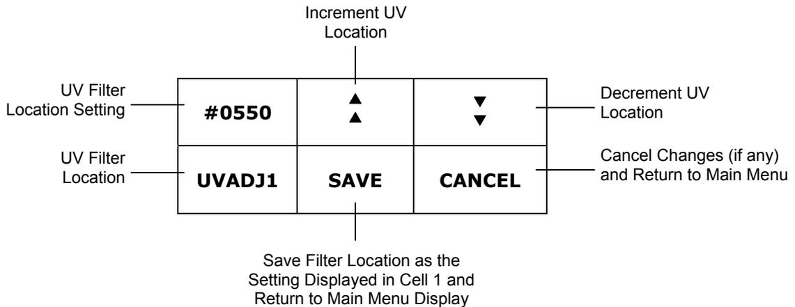
**Figure 3-2. Touch Pad UV Filter Setup Display**
