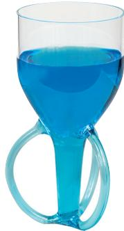
**Rosette Cell:** Branson's Rosette Cell provides a unique flow pattern of substances for exposure to ultrasonic energy during circulation through the cell. When it is immersed in a cooling bath, the enlarged glass surface area and circulation through the side arms provide an efficient means of heat exchange.
