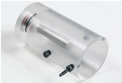
**Cup Horn:** This specialized horn permits high-intensity sound to be applied to multiple samples without direct horn contact. 3.0" diameter only.
