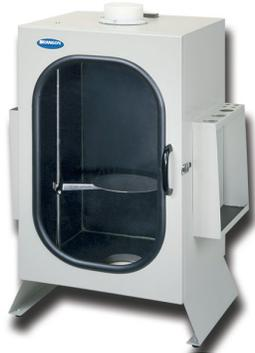
**Acoustic Enclosure:** Operating a Sonifier SFX Series in the Soundproof Enclosure can minimize mechanical noise produced by ultrasonic processing. The sturdy cabinet is lined with waterproof, sound-absorbing material, which is impervious to most solutions or laboratory reagents and can be cleaned easily. A fully-transparent door enables viewing of the process while limiting the noise to an acceptable level.
