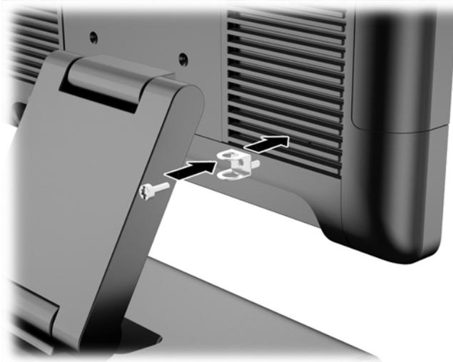
2. Connect a cable that is attached to an external object to the padlock and Insert the padlock into the security loop.
