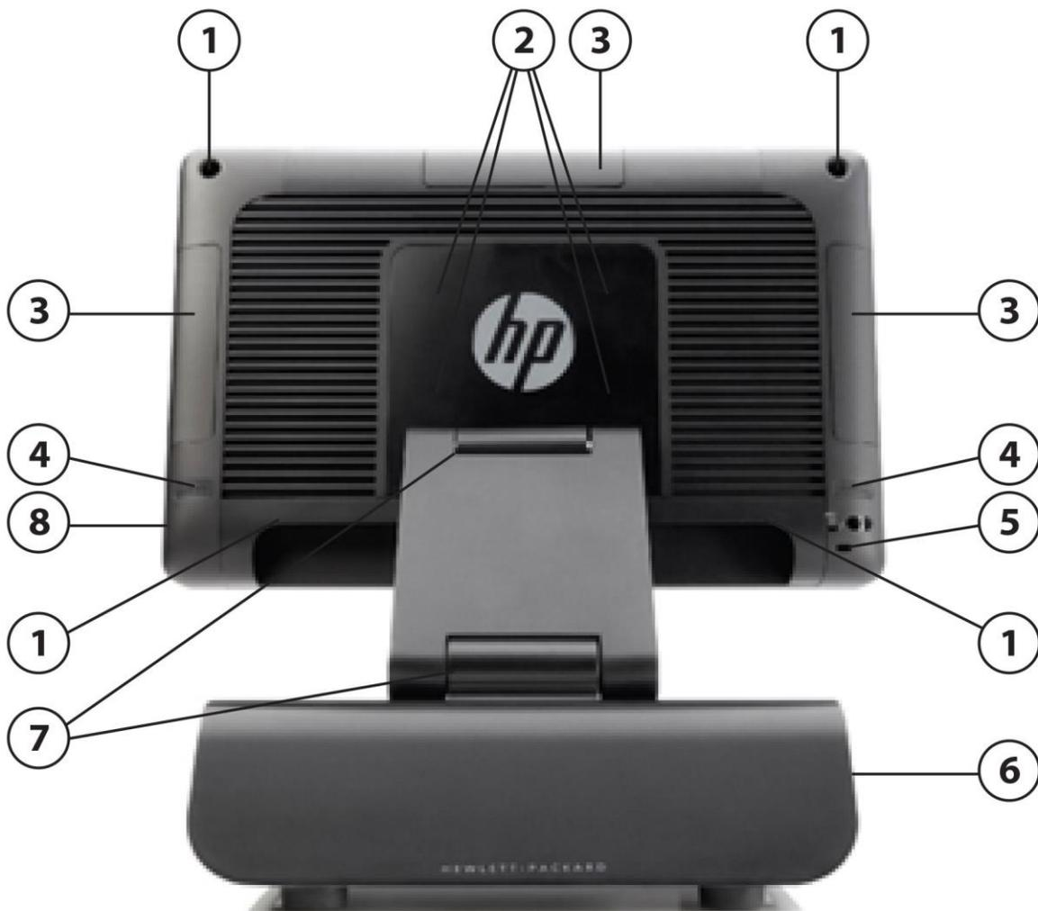
1. Captive Screws (loosen to access core components)
