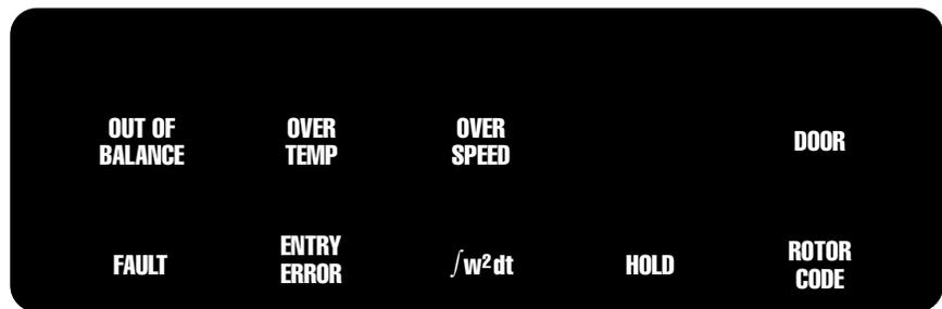
The RC-5C PLUS has nine operator advisory messages on the control panel. These messages are backlit; each message lights only when the condition that it represents exists. The meaning of each message is given below, along with the corrective action.
