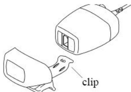
The holder delivered with the sensor can be used to clamp the sensor onto an IV pole or a shelf.
