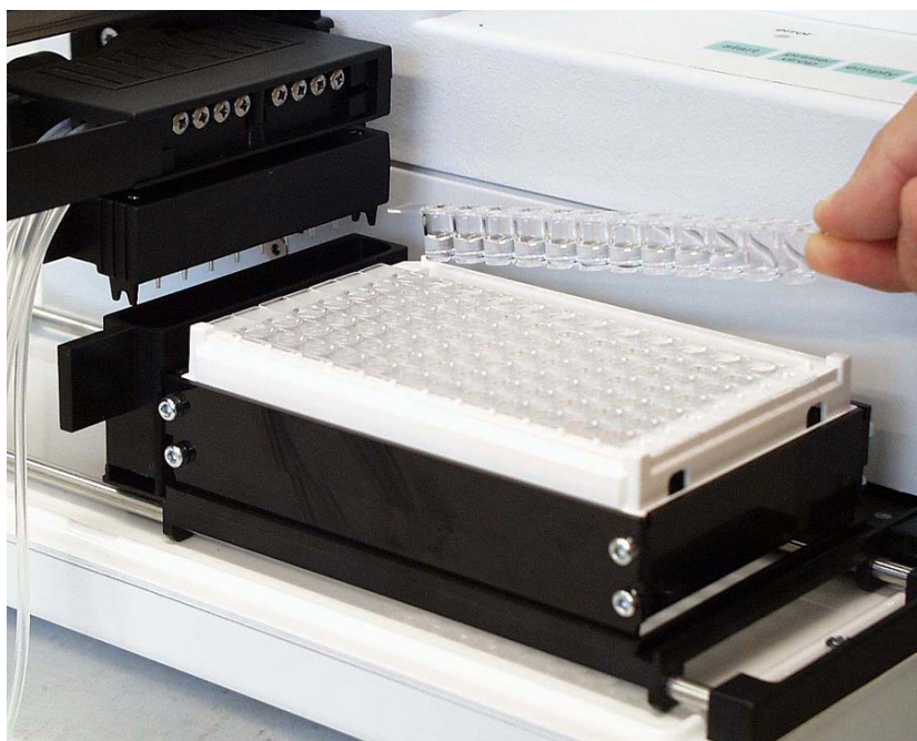
Fig. 7.9 Removing the filled microstrip to be weighed
