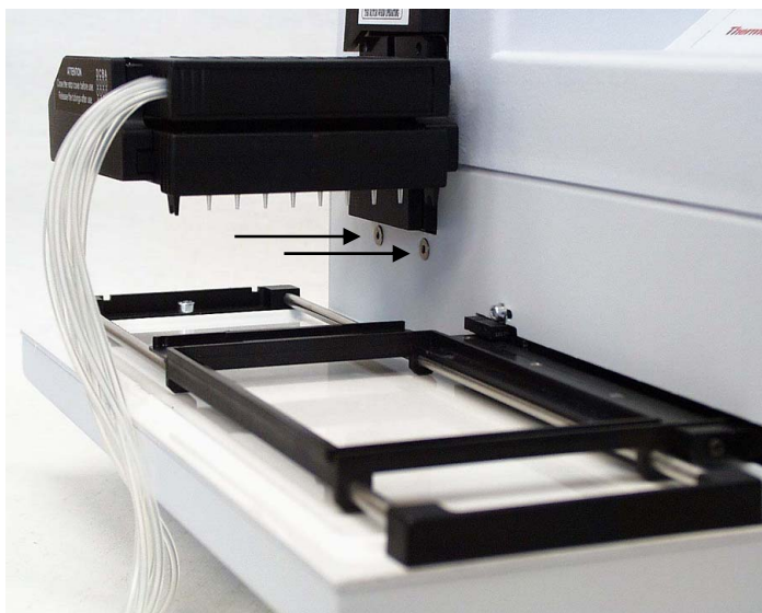
Fig. 6.16 Location of the adjustment screws that may have to be adjusted
