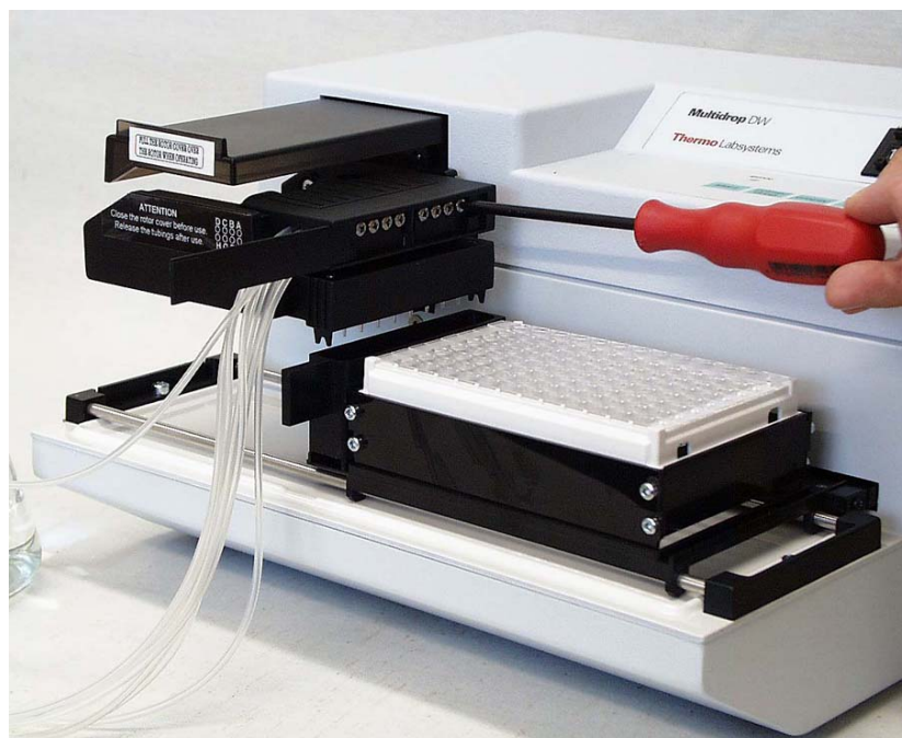
Fig. 7.10 Screwing the calibration screw according to the calibration results
