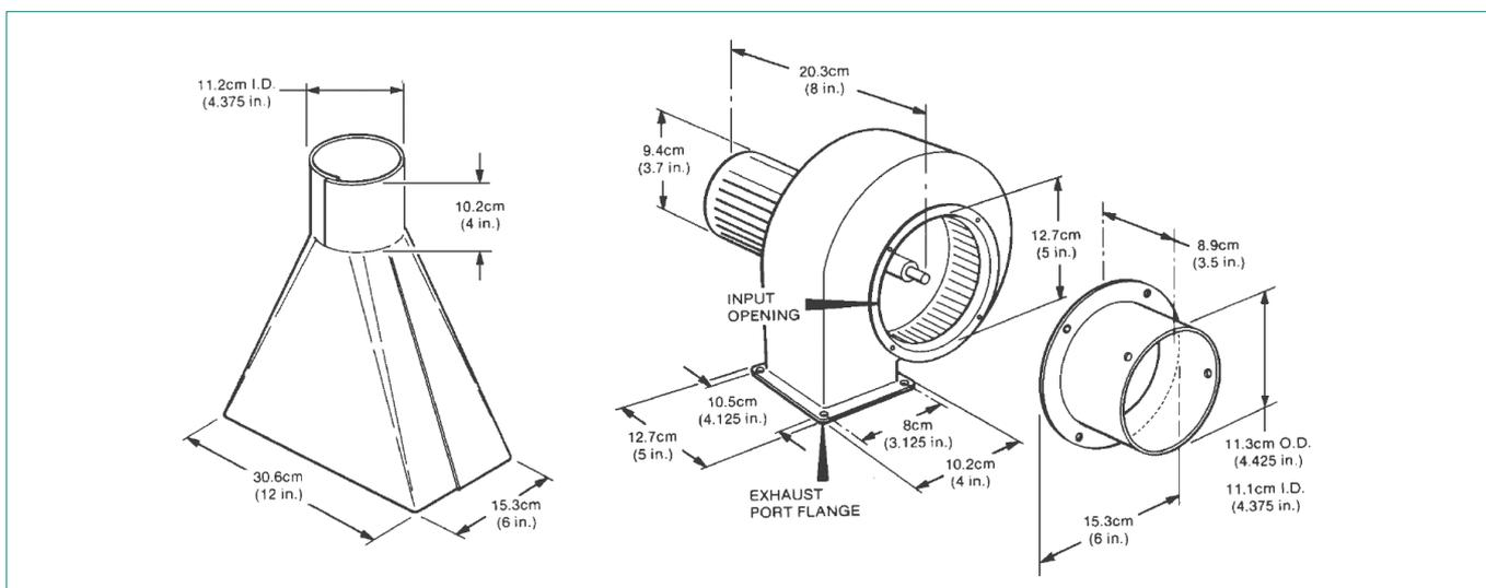
**Figure 1. Blower and vent kit dimensions.**
