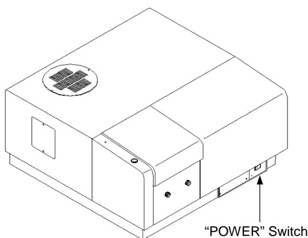
Fig. 2.1 Power switch location
