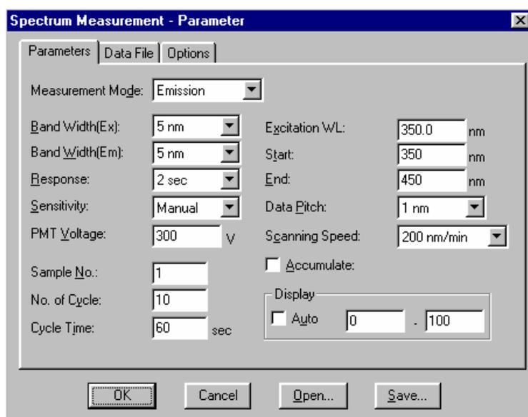
Fig. 5.4 [Spectrum Measurement - Parameters] dialog box(Emission mode)
