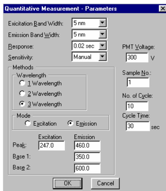
Fig. 4.26 [Quantitative Measurement-Parameters] dialog box
