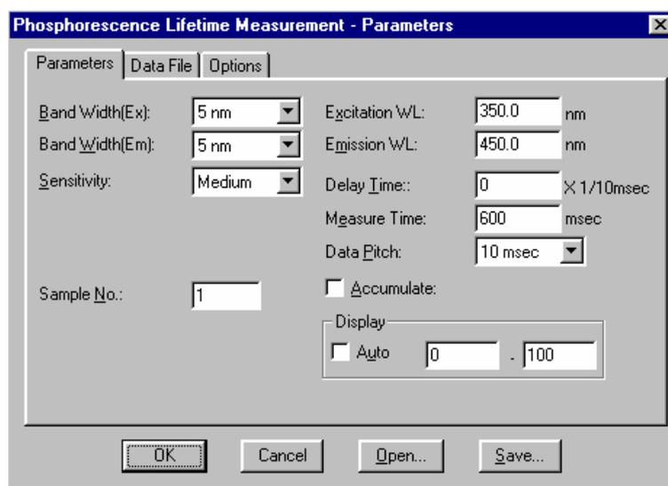
Fig. 10.3 [Phosphorescence Lifetime Measurement - Parameters] dialog box
