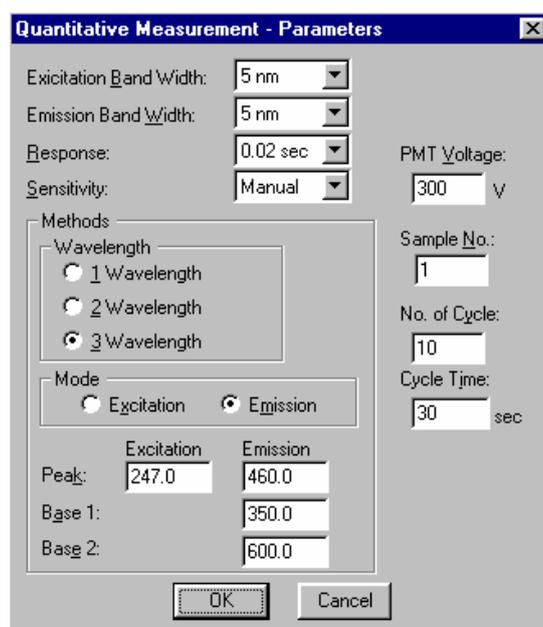
Fig. 3.6 [Quantitative Measurement Parameters] dialog box
