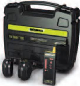
The Tru Pointe® 1100 is a state-of-the-art digital ultrasonic inspection system for leak detection, mechanical inspection and troubleshooting. It accurately detects ultrasounds generated by leaks and pinpoints them at the speed of sound. It detects airborne leaks or electrical arcing in the frequency band of 34 kHz to 42 kHz and 16 kHz to 24 kHz for internal leaks or bearing wear using the patented internal Touch Probe sensor.
