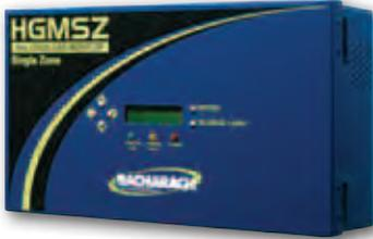
The HGM-SZ (Halogen Gas Monitor Single-Zone) is designed for continuous single-point monitoring of Ammonia, CFC, HFC, HCFC and Halon refrigerant gases. The HGM-SZ displays the type of gas being monitored, along with displaying both the current gas level and the peak gas level detected on its front panel LCD. The instrument retains a log of previous readings that can be easily accessed for analysis.
