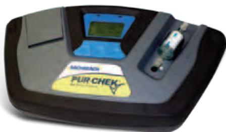
Pur•Chek™ is smarter and faster than any refrigerant identifier used in the industry today. Its compact size and ergonomic design makes testing easy and it utilizes non-dispersive infrared (NDIR) technology to determine the weight concentrations of R12, R134A, R22, hydrocarbons, and air. It also features 'Blend-Chek' analytical software which quickly and accurately indicates the presence of R410A blend refrigerant.
