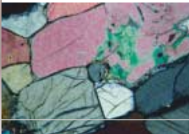
Step 1: orthoscopy, thin section of rock. Center: small olivine crystal.
