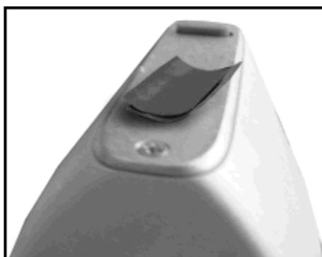
**Figure 19. Correct Way to Measure Heat Shrink Tubing**
