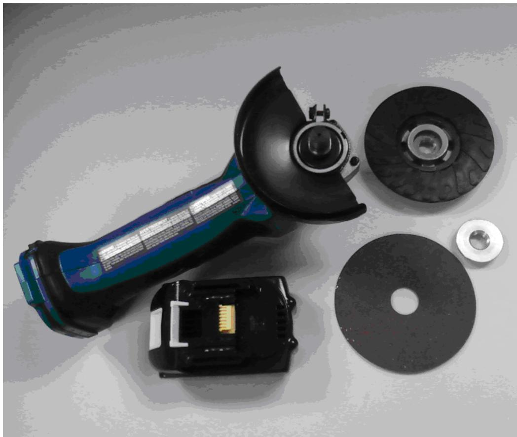
**Figure 7. Assembling the Grinder**
