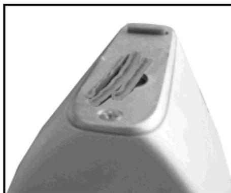
**Figure 17. PVC Wire Insulation With Conductor Removed**
