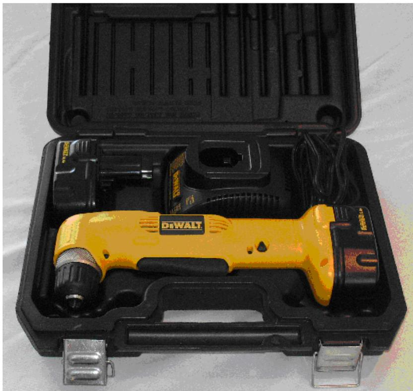
**Figure 1. Example of Right Angle Drill**
