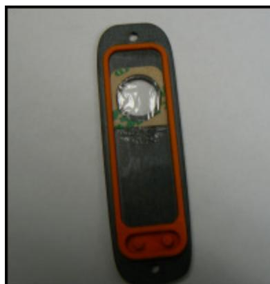
**Figure 6. Measurement Window Replaced**
