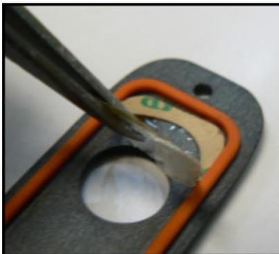
**Figure 2. Removing the Old Window**
