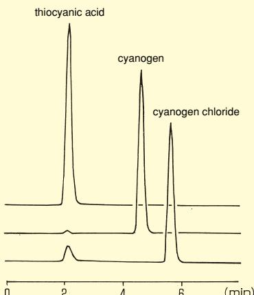
This figure shows the selective results obtained with Shimadzu's unique separation and postcolumn methods, using 4-pyridinecarboxylic acid-pyrazolone. Matrix materials cause almost no interference. Analysis can be performed efficiently in 10-minute cycles; with a high performance column, it takes a mere seven minutes to study a specimen.
