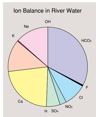
As the VP Series Ion Chromatograph accurately measures bicarbonate ions, it can verify ion balance. This graph indicates accurate data because equal equivalents of anions and cations were exchanged.
