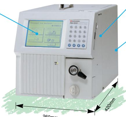
The compact design incorporates both a data processor and floppy disk drive. Even better, with its 2 mm i.d. semi-micro column, this system consumes one-fifth of the solvent used by the 4.6 mm i.d. column.
