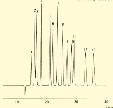
The innovative Shimadzu postcolumn pH-buffered conductivity detector aids in high sensitivity, selective analysis of organic acids. Most samples, even those once demanding extensive pretreatment to eliminate matrix components, only require simple dilution or filtration for analysis. Furthermore, the organic acid analysis System can also study inorganic weak acids, including silicic, boric, cyanic, and carbonic acids.
