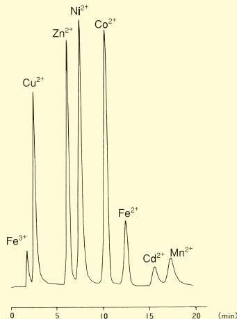
In the transition metal analysis system, PAR [4-(2-pyridylazo)-resorcinol], a reaction reagent in the postcolumn visible absorbance detector, promotes sensitive selective analysis of transition metals. Furthermore, after a system upgrade, the arsenazo III reagent can be used in the selective analysis of rare-earth metal ions.
