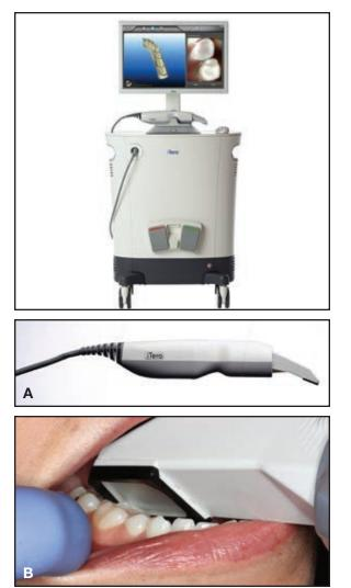
Fig. 5 A. iTero intraoral scanner with sealed keyboard, wireless mouse, and wireless foot pedal; parallel confocal imaging enables powder-free scanning. B. Wand held at 45° to capture both lingual and occlusal surfaces.
