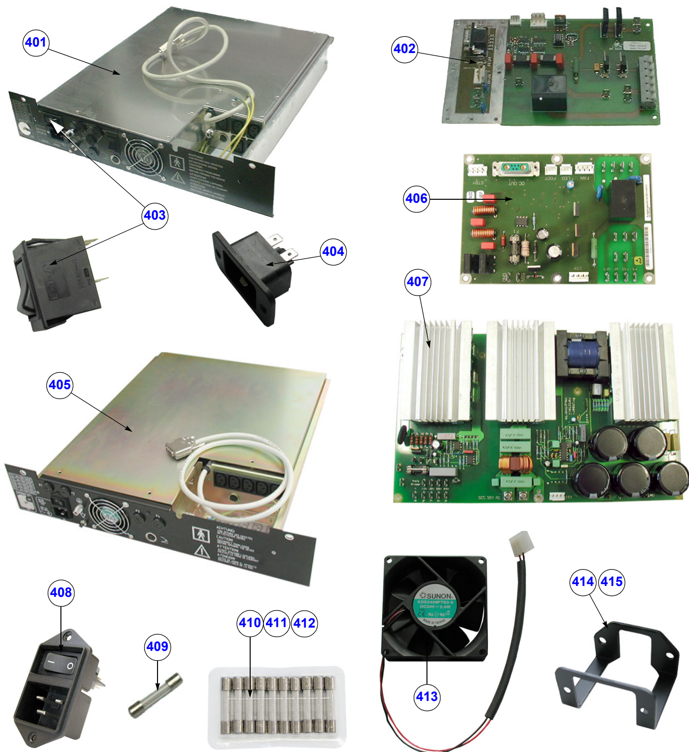
Figure 9-7 Main Power Module (CPN)
