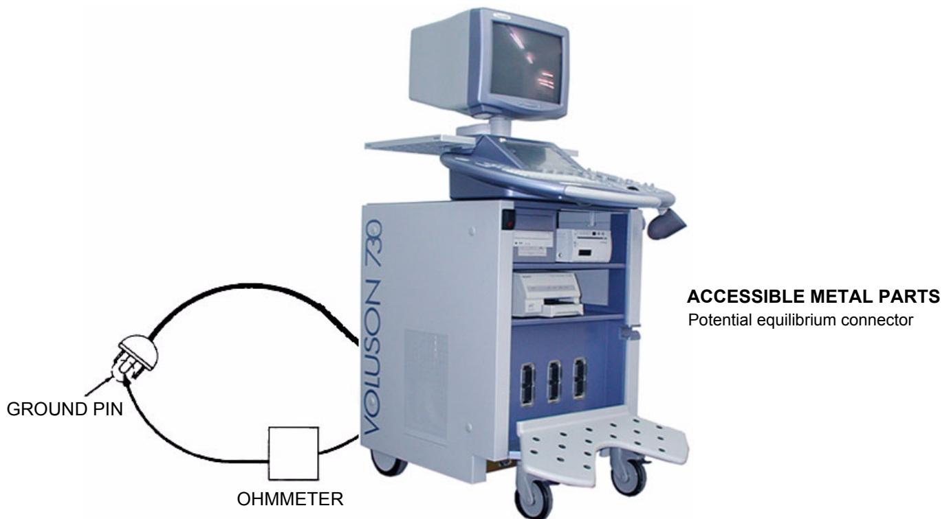
Figure 10-2 Ground Continuity Test
