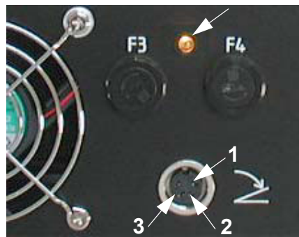
Figure 7-2 Diagnostic LED's and corresponding voltage check points
