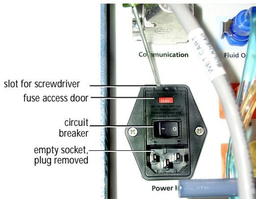
Removing the plug allows easier access to the fuse door.
