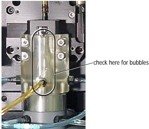
If you see bubbles, remove them as described in *Removing Bubbles from the Flow Cell* on page 115.
