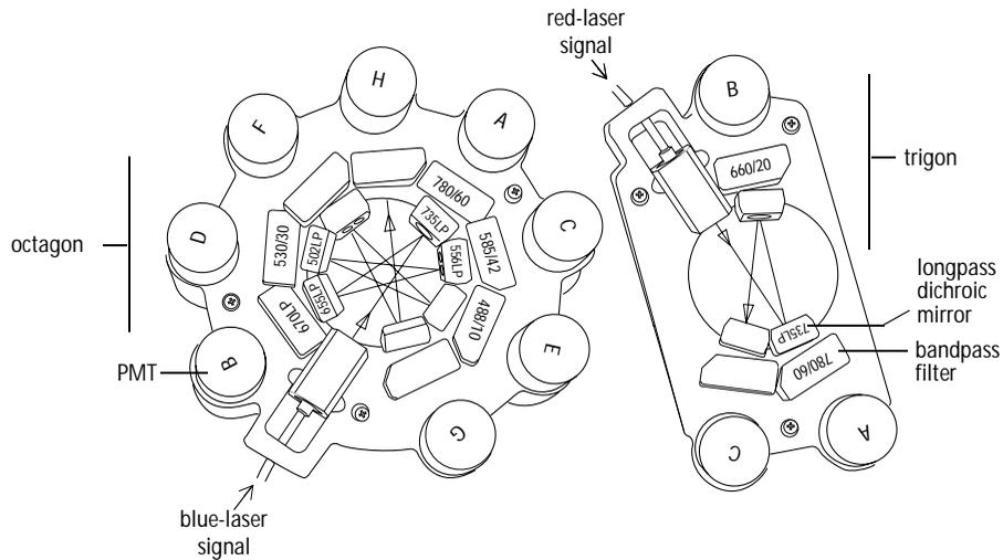
When light arrives at an array, a long-pass dichroic mirror transmits the highest wavelengths to the first PMT in the series and reflects lower wavelengths to the next PMT. Likewise, the next PMT's long-pass dichroic mirror will transmit the next highest wavelengths and reflect lower wavelengths, and so on around the array. A bandpass filter in front of each PMT further screens unwanted light.
