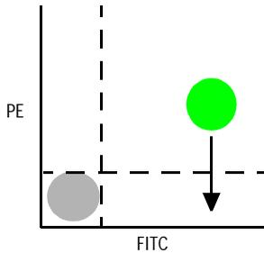
If the fluorescence is to be assigned to PE, the FITC signal must be removed from the PE channel, as indicated by the arrow. Both PE and FITC fluoresce in the yellow (575 nm) range, so there is no way to isolate the emission from each fluorochrome optically. Instead, fluorescence compensation moves the FITC population out of the PE positive area (Figure A-13).
