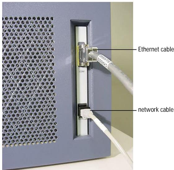
Both cables connect to ports on the PC workstation. As the make and model of the workstation might vary, refer to the documentation that came with your system for information.
