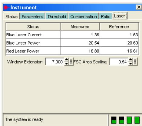
The Laser tab also contains Window Extension and FSC Area Scaling controls. The Window Extension extends the time in which area is measured. The FSC Area Scaling factor adjusts area measurements to be on the same scale as height measurements for signals from the FSC photodiode.
