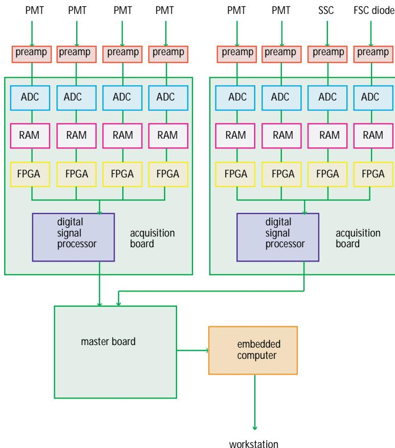
The pulse is amplified and then sent to a 14-bit analog-to-digital converter (ADC) on the acquisition board that changes the analog (continuous) pulse into digital (discrete) data. The ADC does this by sampling the pulse up to 10 million times per second, slicing it into 16,384 levels, and assigning a measurement to each time sample (Figure A-17 on page 166).
