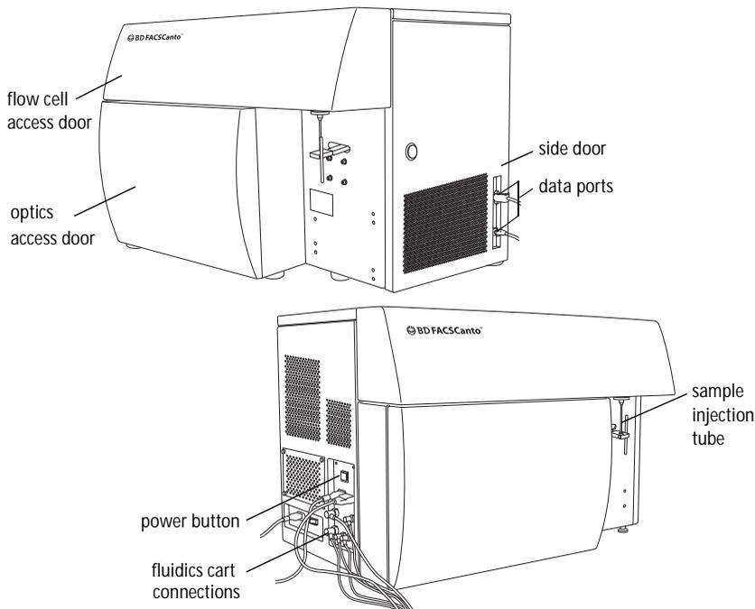
The BD FACSCanto flow cytometer consists of an optics subsystem, a fluidics subsystem, and an electronics subsystem. For a more in-depth discussion of fluidics, optics, electronics, and flow cytometry, see the Technical Overview on page 149.
