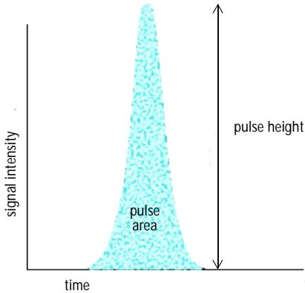
An FPGA calculates pulse height and area in the following manner:
