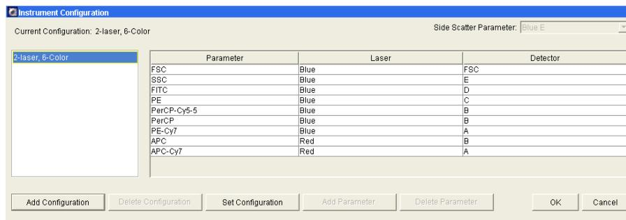
Before you start any Experiment, verify that the instrument configuration contains appropriate parameters for the samples you are running, and that the instrument optics match the current configuration. If needed, you can define a custom configuration for your system setup and application.
