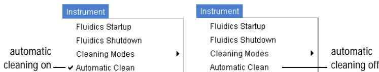
When automatic cleaning is on (command checked), the system runs Fluidics Startup automatically each time a user logs in or the cytometer resumes running from Standby, and runs Fluidics Shutdown each time a user logs out or the cytometer is put into Standby.
