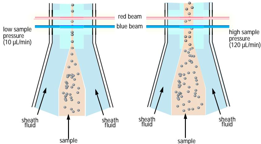
When using BD FACSCanto clinical software, the cytometer automatically regulates the sample pressure according to the currently selected panel.
