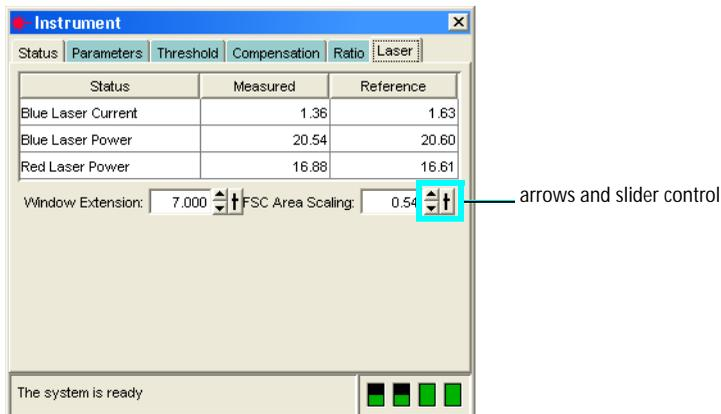
Adjust the value until the events in the plot are approximately at a 45 degree angle.
