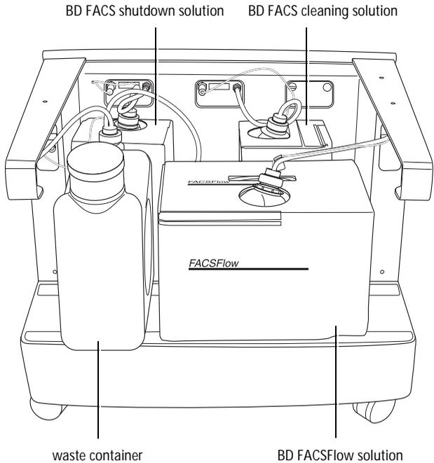
Each cubitainer and the waste tank has its own port. Connect the cubitainers and waste tank to the ports listed in the following table.
