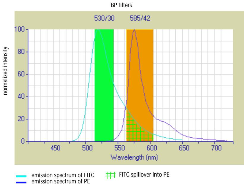
For example, FITC appears primarily in the FITC detector, but some of its fluorescence spills over into the PE detector. PE appears primarily in the PE detector, but some of its fluorescence spills over into the FITC detector. This spillover must be corrected, or compensated, for. Thus, the term compensation.
