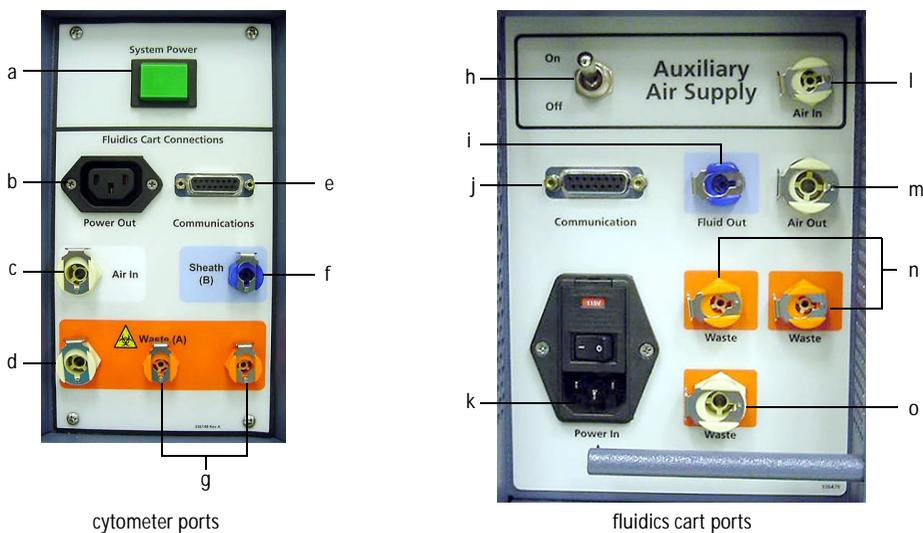
The ports on the cytometer have their corresponding fluidics cart ports listed in Table 4-2. For example, make sure the tubing for *f. Sheath (B)* connects to the port labeled *i. Fluid Out*. Table 4-3 on page 127 lists port functions.
