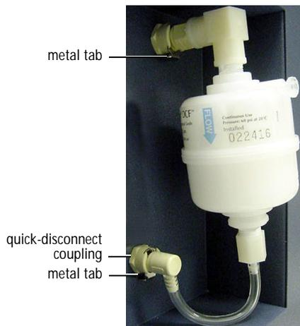
**3** Install the bypass tubing in place of the filter.
