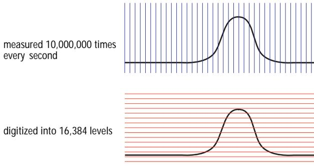
The ADC sends these numbers to short-term memory (RAM) so that a field programmable gate array (FPGA) can rebuild a digital version of the pulse for analysis.
