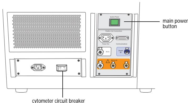
The instrument circuit breaker is located next to the power cord (Figure 1-6). The breaker will need to be reset if there is a power surge in the laboratory.
