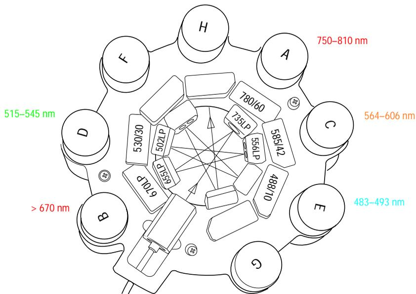
Behind the LP mirror, a 780/60 BP filter admits light from 750 nm to 810 nm and substantially blocks other wavelengths. The light that finally reaches PMT A will from dyes such as PE-Cy7 that emit in this range.
