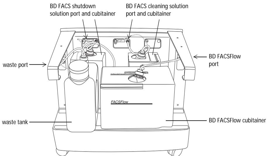
Each solution has its own non-interchangeable fluid port and level-sensor connection. Fluid level alarms occur within BD FACSCanto clinical software and BD FACSDiva software.
