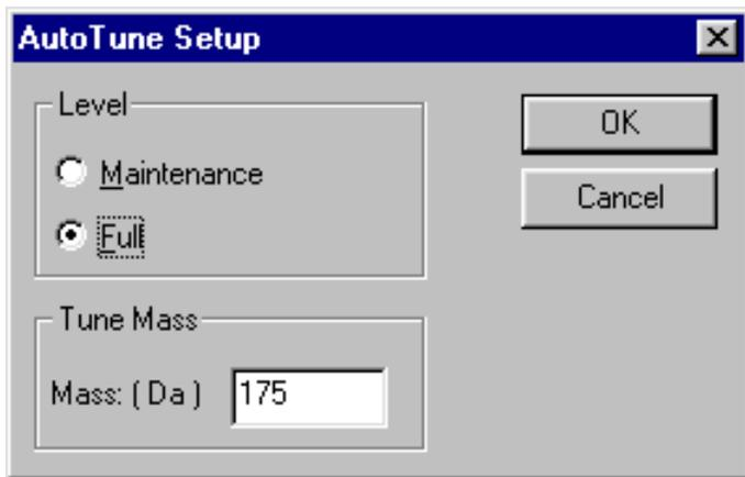
The Tune Mass parameter sets the mass to be tuned on.
