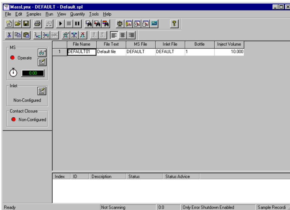
4. Select Options from the menu bar, then Pump. The rotary pump starts to evacuate the detector. In about 20 minutes, the instrument is sufficiently evacuated to enable operation, and the Vacuum indicator on the front panel shows green.
