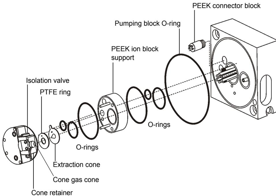
21. Place the ion block on a flat surface, and remove any O-rings.
