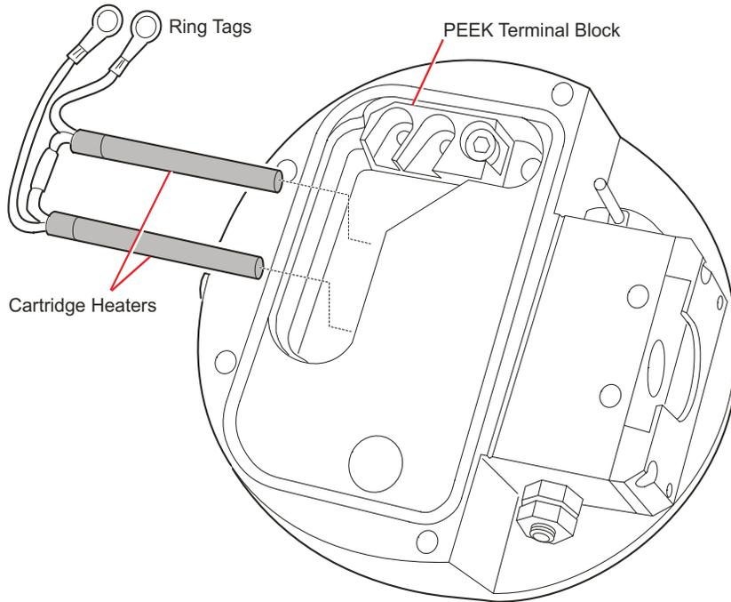
4. Loosen the two set screws that secure the heater cartridges in the ion block, using the 1.5-mm hex wrench.
