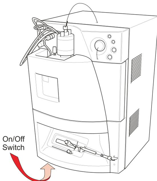
2. Allow 3 minutes for the embedded PC to initialise. An audible alert is given when the PC is ready.
