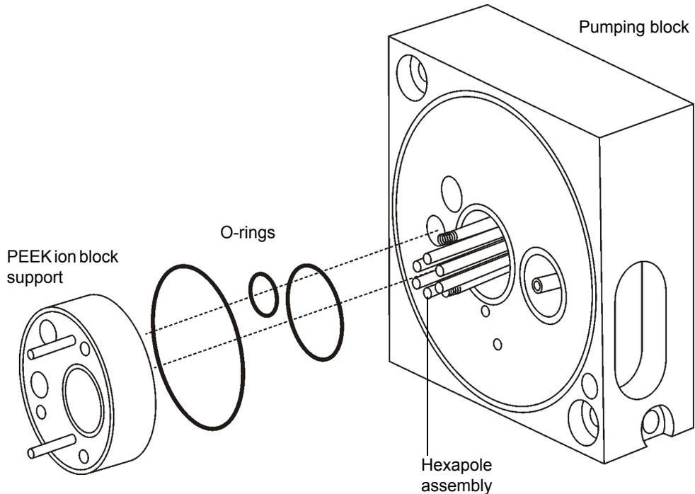
2. Remove any O-rings that remain stuck to the surface of the pumping block.
