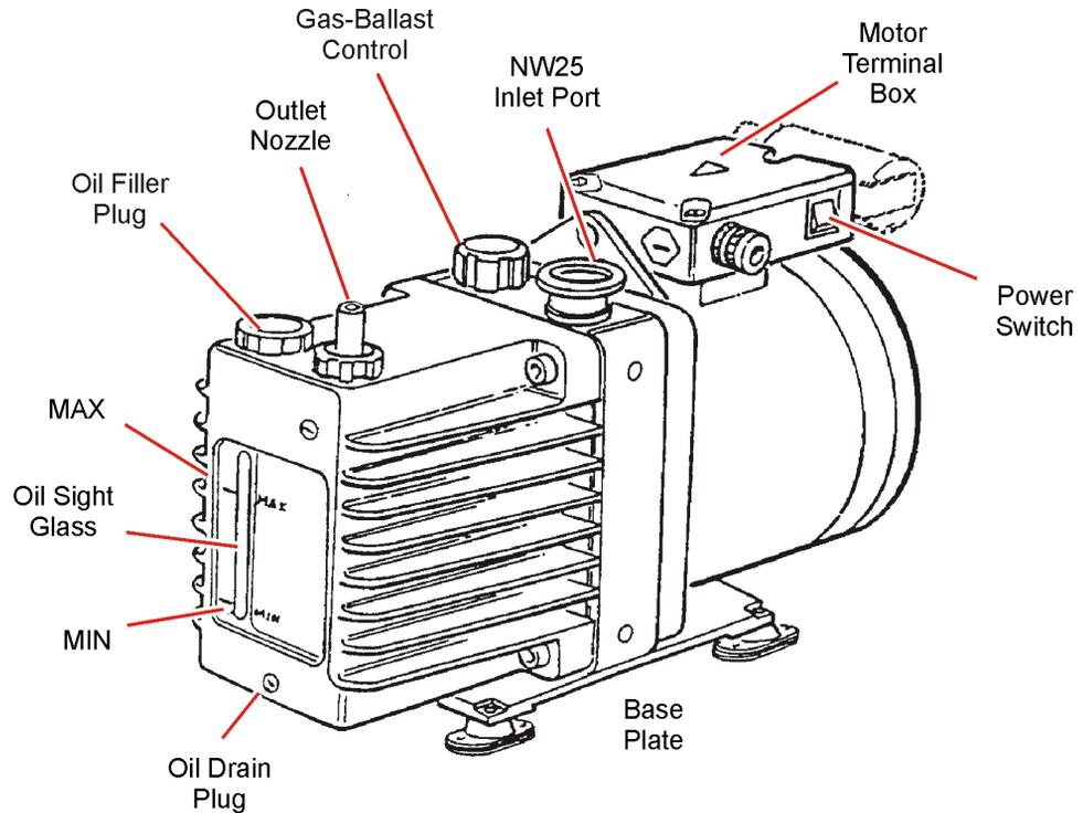
3. When the oil is clear and has drained back to the rotary pump, return the gas-ballast control to its normal position.
