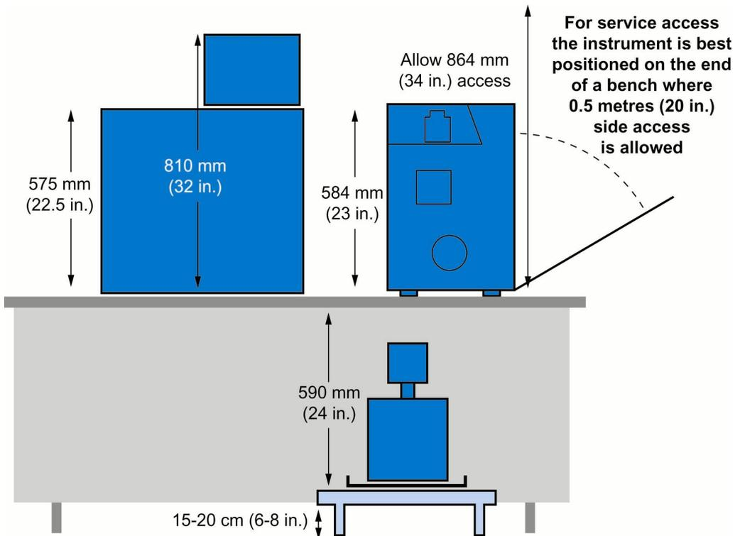
Ideally, the following minimum clearances should be allowed for service access and ventilation:
