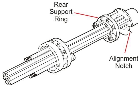
5. Carefully suspend the hexapole assembly in a graduated cylinder, then add methanol to the cylinder until the assembly is covered.
