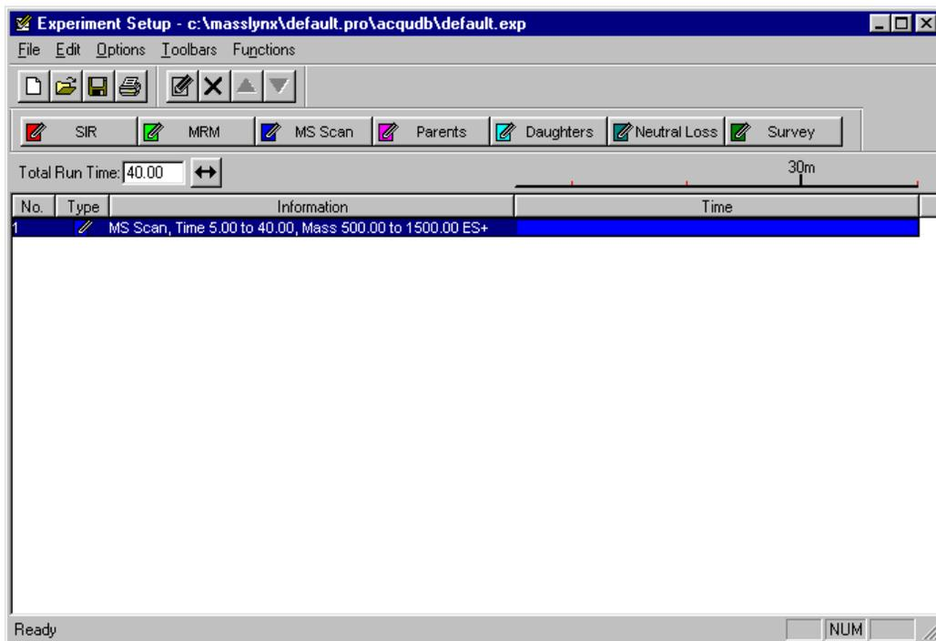
The figure above shows a simple function list containing only one function: a centroided mode full scan, between 500 and 1500 amu using ES+ ionization. Immediately above the function bar display is a time scale that shows from when the function is active, and for how long it runs. In this case, the function starts after 5 minutes and then runs for 35 minutes, terminating after a total elapsed time of 40 minutes.
