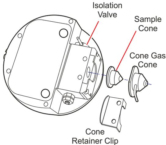
17. Carefully separate the sample cone from the gas cone, then remove the sample cone O-ring.
