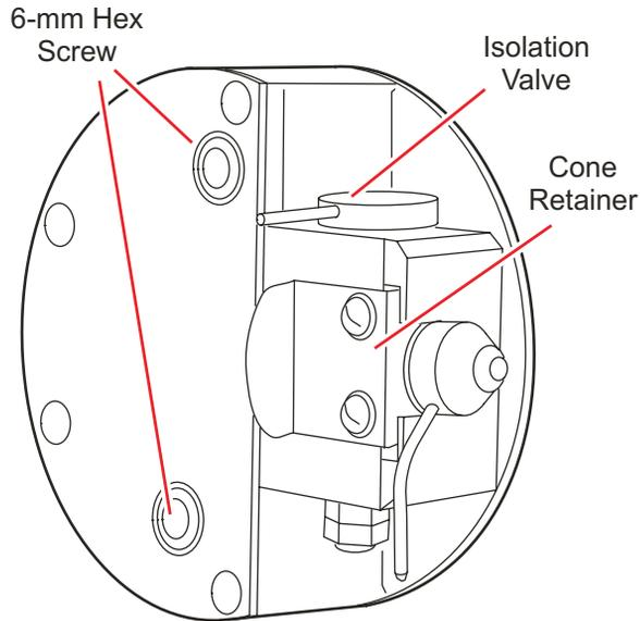
16. Remove the cone gas cone, O-ring, and sample cone from the ion block.
