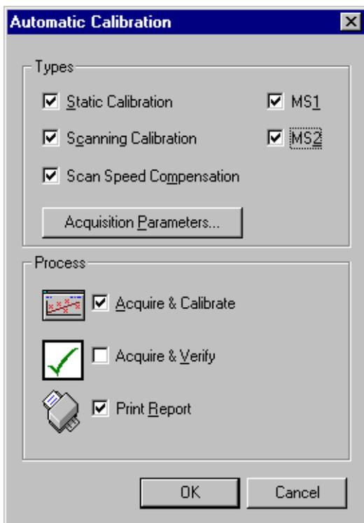
It is recommended that all three types of calibration are performed so that mass ranges and scan speeds can be changed whilst maintaining correct mass assignment. However, it is possible to have any combination of these calibrations:
