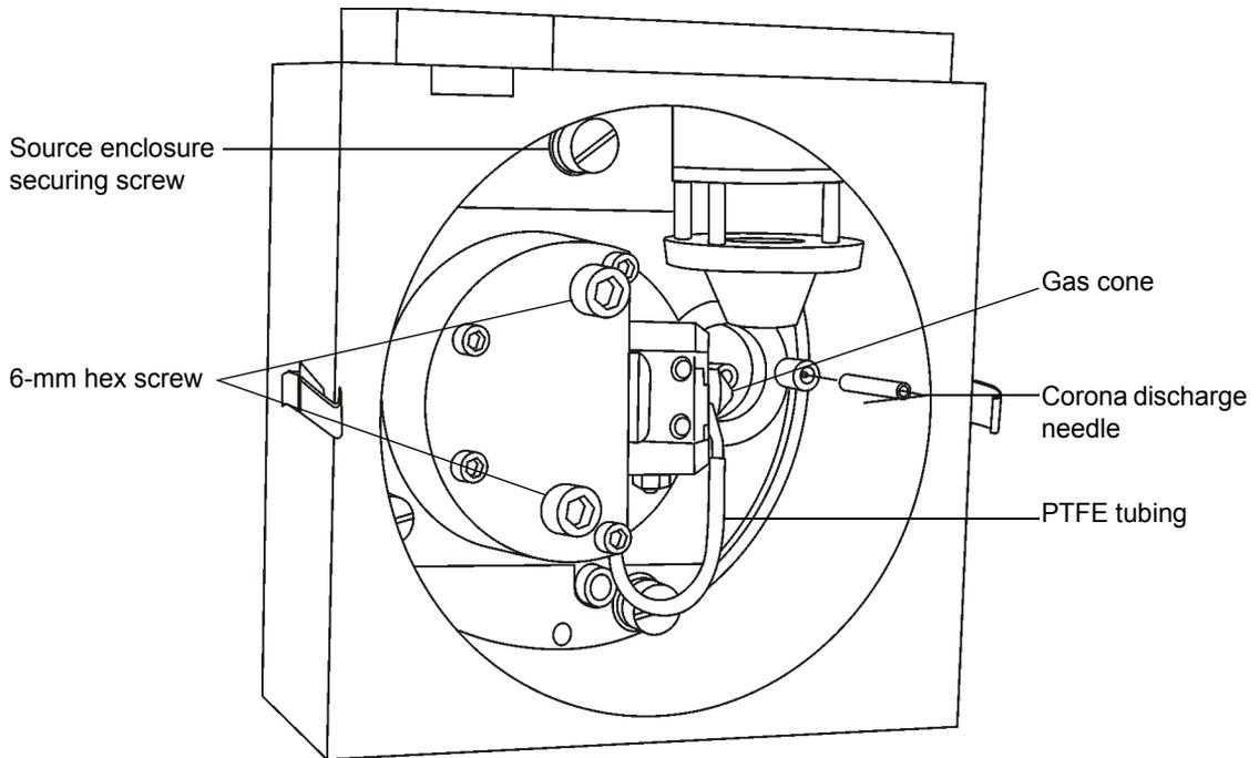
14. Remove the PTFE tube attached to the cone gas cone.
