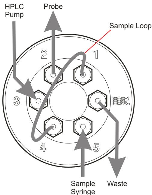
The divert/injection valve is an electrically driven Rheodyne<sup>®</sup> injector that may be used in several ways depending on the plumbing arrangement:
