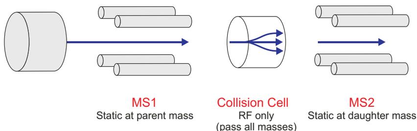
This mode is the MS/MS equivalent of SIR (Selected Ion Recording). As both MS1 and MS2 are static, this allows greater dwell time on the ions of interest and therefore better sensitivity compared to scanning MS/MS.
