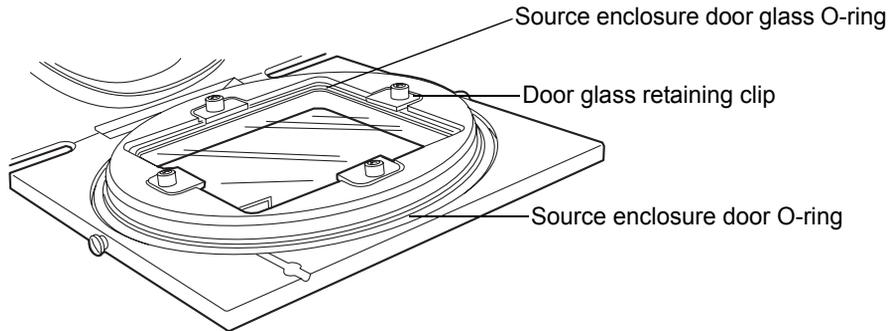
6. Use a hex (Allen) key to remove the four bolts securing the source enclosure door glass retaining clips to the source enclosure door.
