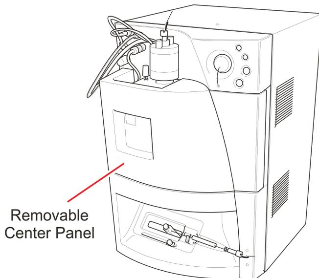
The Quattro™ micro API is a high performance triple quadrupole mass spectrometer designed for routine LC/MS/MS operation.
