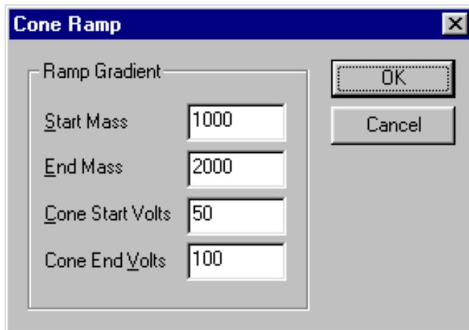
Two values of cone voltage are defined at two particular masses. These values define a gradient for the cone voltage which is then extrapolated to cover the full mass range.
