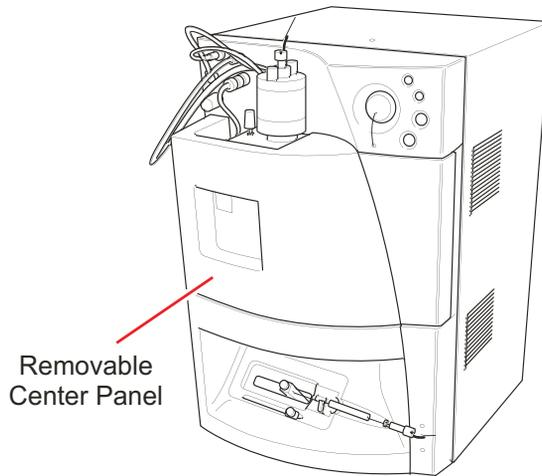
12. Unfasten the source enclosure door's securing clips and open the door.
