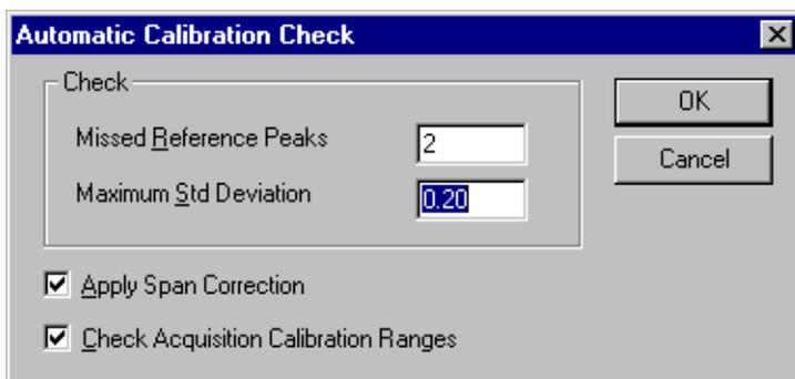
This dialog box defines limits which the calibration must attain before the instrument is successfully calibrated. Two user parameters can be set:
