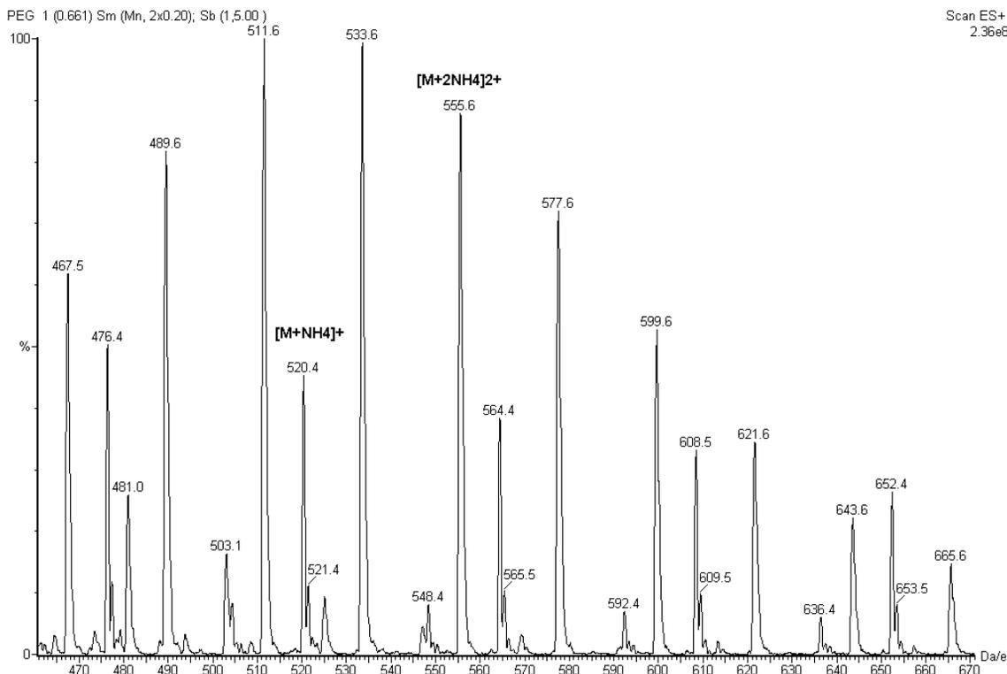
A low Cone voltage encourages the production of doubly-charged ions. The voltage should be at least 35 V.
