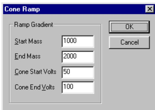
The four parameters define a gradient for the cone voltage which is then extrapolated to cover the full mass range of the function.
