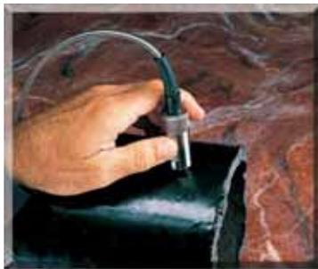
You can now forget the time-consuming removal of coatings. The TopCOAT function of the DMS 2TC helps to measure not only the thickness of the base metal, but at the same time also that of the coating layer. Moreover, you'll have other possibilities of measuring through coatings at your disposal under certain conditions, e.g. measurement within the echo sequence (Dual-Multi function).
