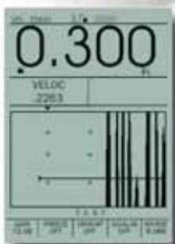
left: A-scan with large-digit display of the measured value
