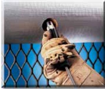
Thickness measurements on hot components are no problem with the DMS 2. We have different dual-element probes in our delivery program allowing to reliably measure components at high temperatures up to 600 °C, including coupling monitoring.
