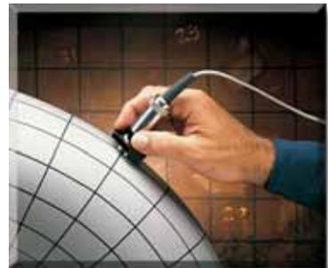
Using the Auto-V function, you can now measure components with unknown material velocity – without any previous comparison measurement by mechanical means! Other advantages: measuring errors in the case of material velocity variations due to temperature variations – e.g. with plastic materials – or due to inhomogeneous materials – e.g. grey cast iron – are eliminated; testing reliability therefore increases.
