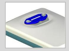
After inserting the strip, apply a small amount of finger pressure to ensure the elastomer is seated squarely in the slot.
