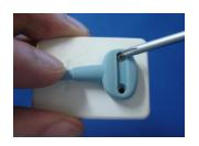
Using the screwdriver provided, loosen and remove the 2 screws that secure the cable to the Sensor. Dispose of the screws as new ones are supplied. Remove the cable from the Sensor.
