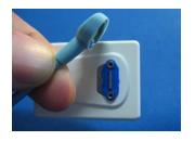
Remove cable from kit. Align the cable to the Sensor so the Sensor keying feature connects to the corresponding key in the cable. When properly aligned, the cable fits the back of the Sensor evenly and the metal area is completely covered.
