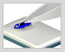
Using a tweezers, take a new (blue) strip from the CDR Elite spare parts kit and insert the strip into its slot in the Sensor. Strip shown darker in this image for clarity.
