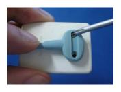
Using the screwdriver, tighten the first screw just until you feel some resistance. Repeat this action for the second screw. Fully tighten both screws and make sure that they are securely tightened.
