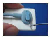
Using a dental instrument, carefully lift and remove the tab cover from the back of the Sensor cable. Dispose of the tab cover as a new one will be used when the new cable is attached.
