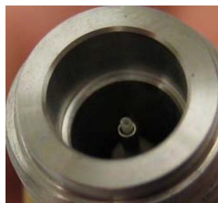
Sample line installed correctly
