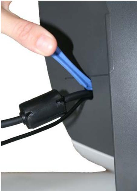
3. Connect the main power cable and the USB cable to the scanner and close the cable compartment cover.
