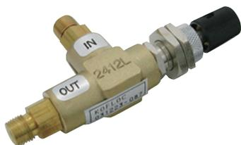
This valve is used to control the gas flow rate. The control range is 0 - 0.7L/min for nitrogen under an inlet pressure of 300 kPa. Shimadzu M type joints are used at both the inlet and outlet.
