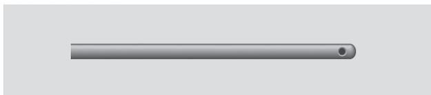
Samples are filled and dispensed through the side hole, eliminating septum plugging of the needle. Ideal for large-volume gas injections. The solid domed tip minimizes septum damage.
