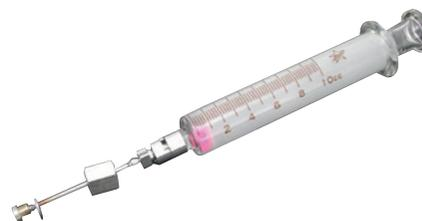
This is a 10 mL syringe with an M type joint. It is conveniently used to wash the inside of a tube with a solvent.
