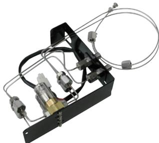
This Solenoid Valve Unit is connected to the detector's supply gas (hydrogen, air). It not only can shut off the supply gas according to instrument power supply or system ON/OFF operation, but also enables automatic start up and shutdown after analysis ends. Therefore, the supply gas can be shut off during a power outage to ensure a safer laboratory. Flame status can also be monitored in GC-2014.
