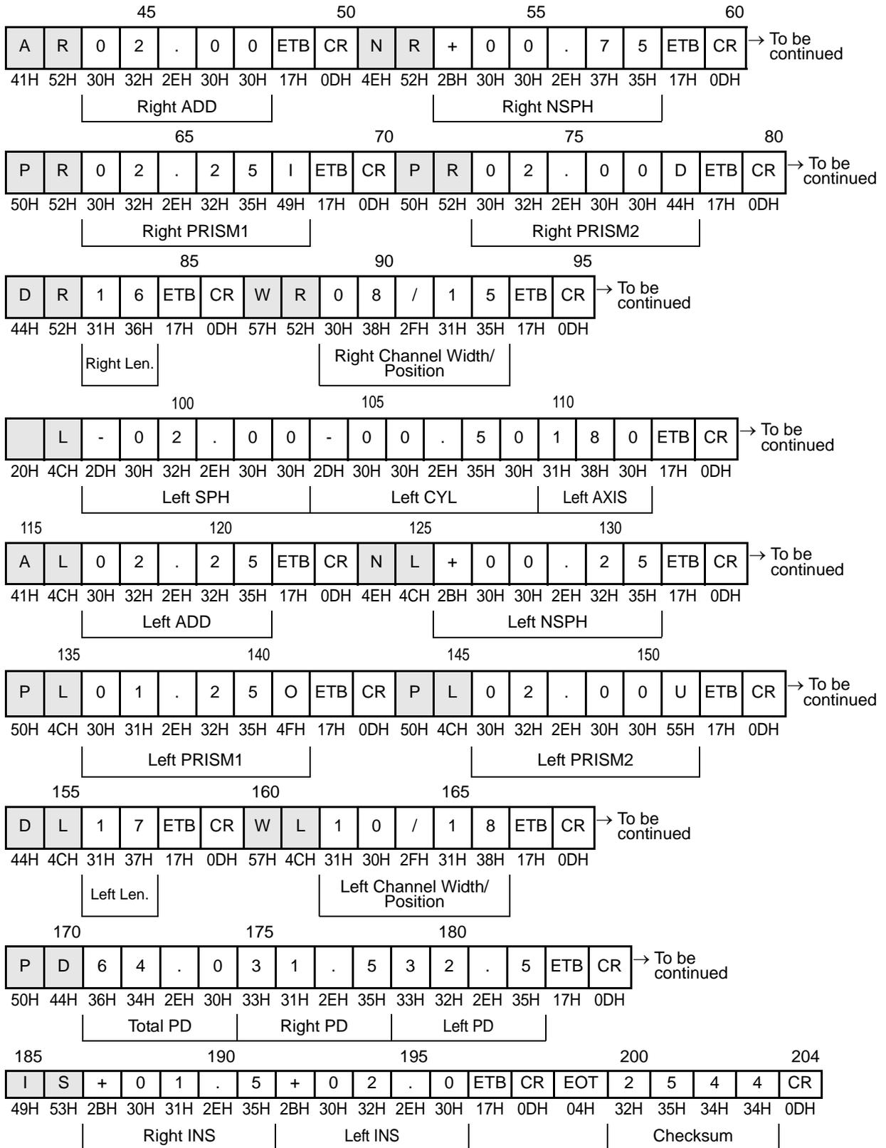
**(14) In the case of the maximum data size in contact lens measurement mode**
