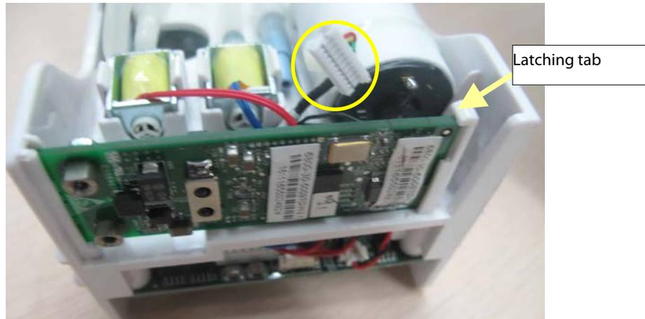
4. Disconnect the cables of the NIBP inflation pump and the relief valves from the parameter board. Snip off the cable ties to remove the pump. Release the tabs to remove the valves.
