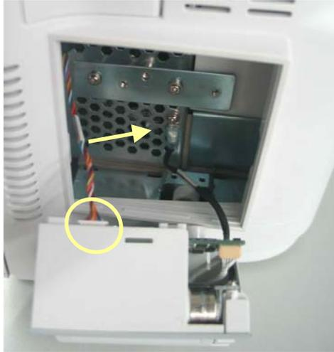
4. Pull the two clips backwards and remove the recorder driving board.
