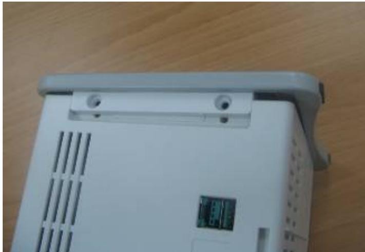
3. From the left side, remove the cable that connects the SMR interface board and the SMR communication board. Then take out the SMR from its housing.
