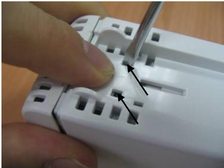
4. Remove the contact screws, the spanner, and the front cover by referring to steps 1 to 3 as described in section **6.5.1 Disassembling the BeneLink Module**.
