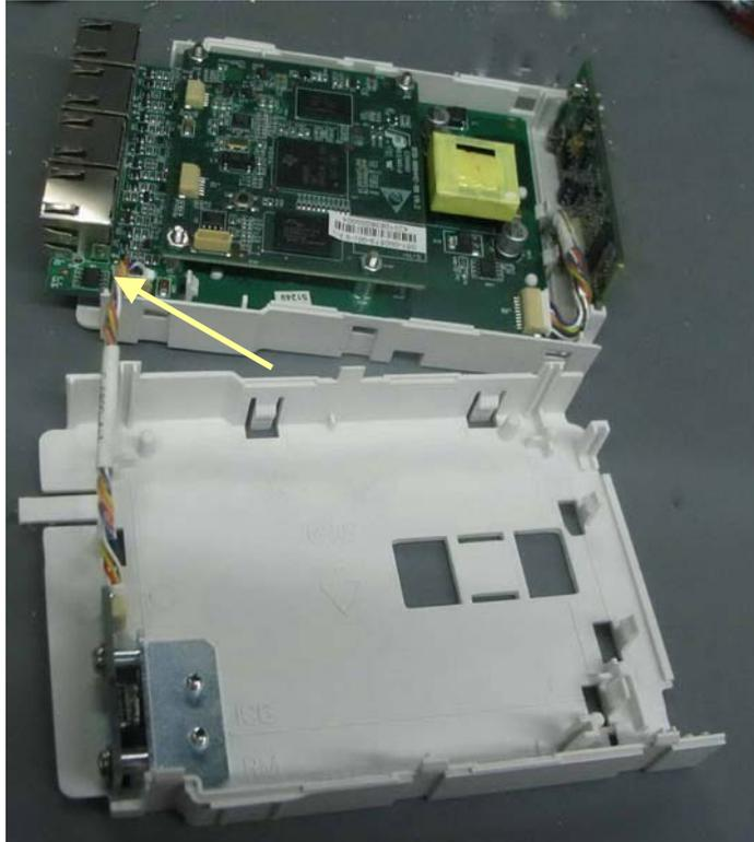
8. Take off the cable between the infrared communication board and the interface board to remove the infrared board.
