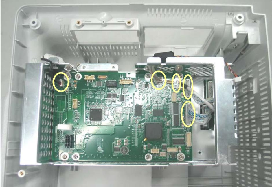
2. Unscrew the 4 M3×6 screws and take out the main board assembly.
