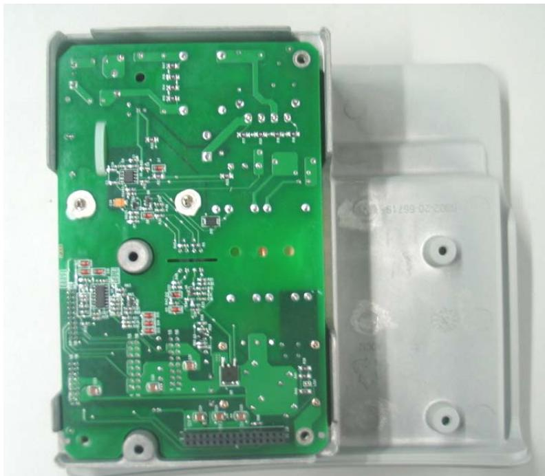
4. Unplug the cable between the AC input filter and the power board, then remove the power board.
