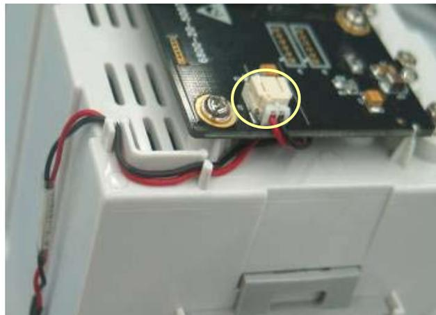
6. Release the clips and take out the Nios II module. Then unscrew the six M3x6 screws and remove the SMR communication board.
