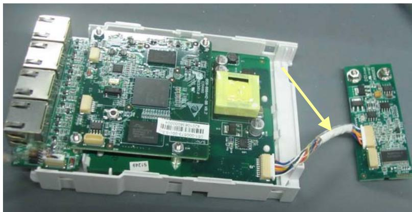
9. Unclench the four clips with a tweezer to remove the interface board.
