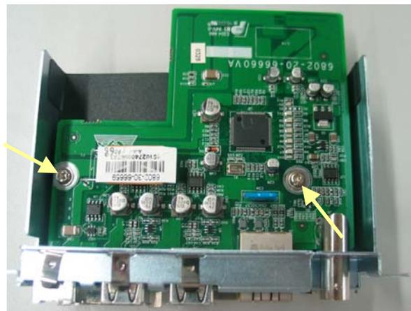
4. Remove the insulating pad from the interface board. Unscrew the two M3×6 screws on the DVI interface board. Then unscrew the two screws beside the DVI socket, the two screws beside micro-D socket and the two M2.5×6 screws.
