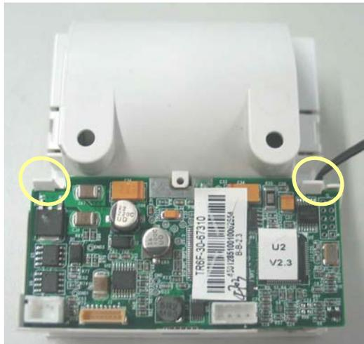
5. Pull the press bar upwards about 1 mm and then unplug the flexible cable. Remove the cable that connects the driving board and the button board. Unscrew the PT2x6 screw and remove the drive board's grounding cable. Then take out the recorder driving board.
