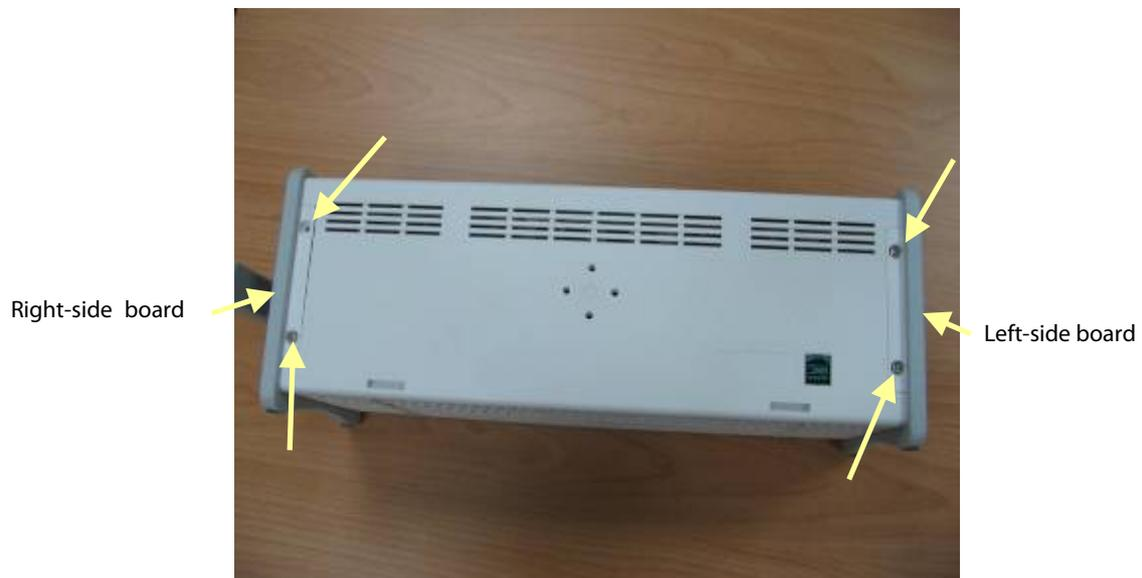
2. Pull the left- and right-side boards outwards. Be sure to place the rubber ring in position when reassembling the right-side board.
