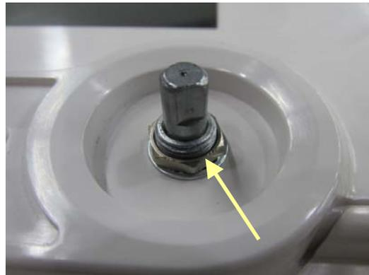
2. Disconnect the cable that connects the knob encoder and the button board to remove the knob encoder.
