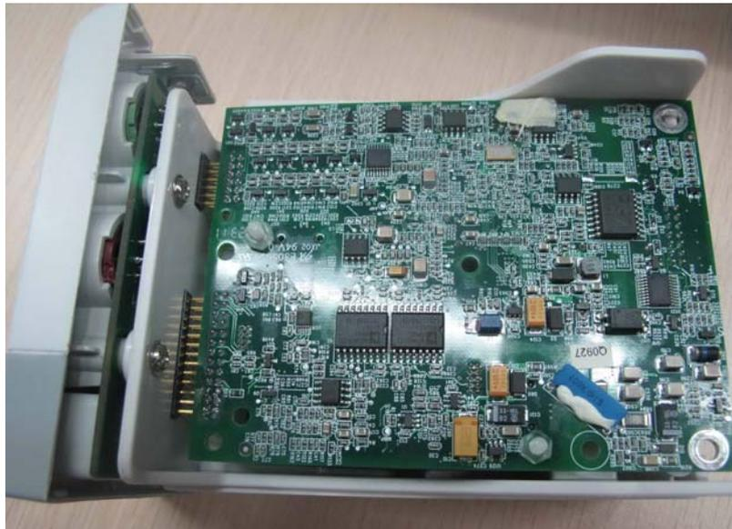
6. Remove the two M3×4 screws on the SpO<sub>2</sub> board to separate the SpO<sub>2</sub> board and the parameter board.
