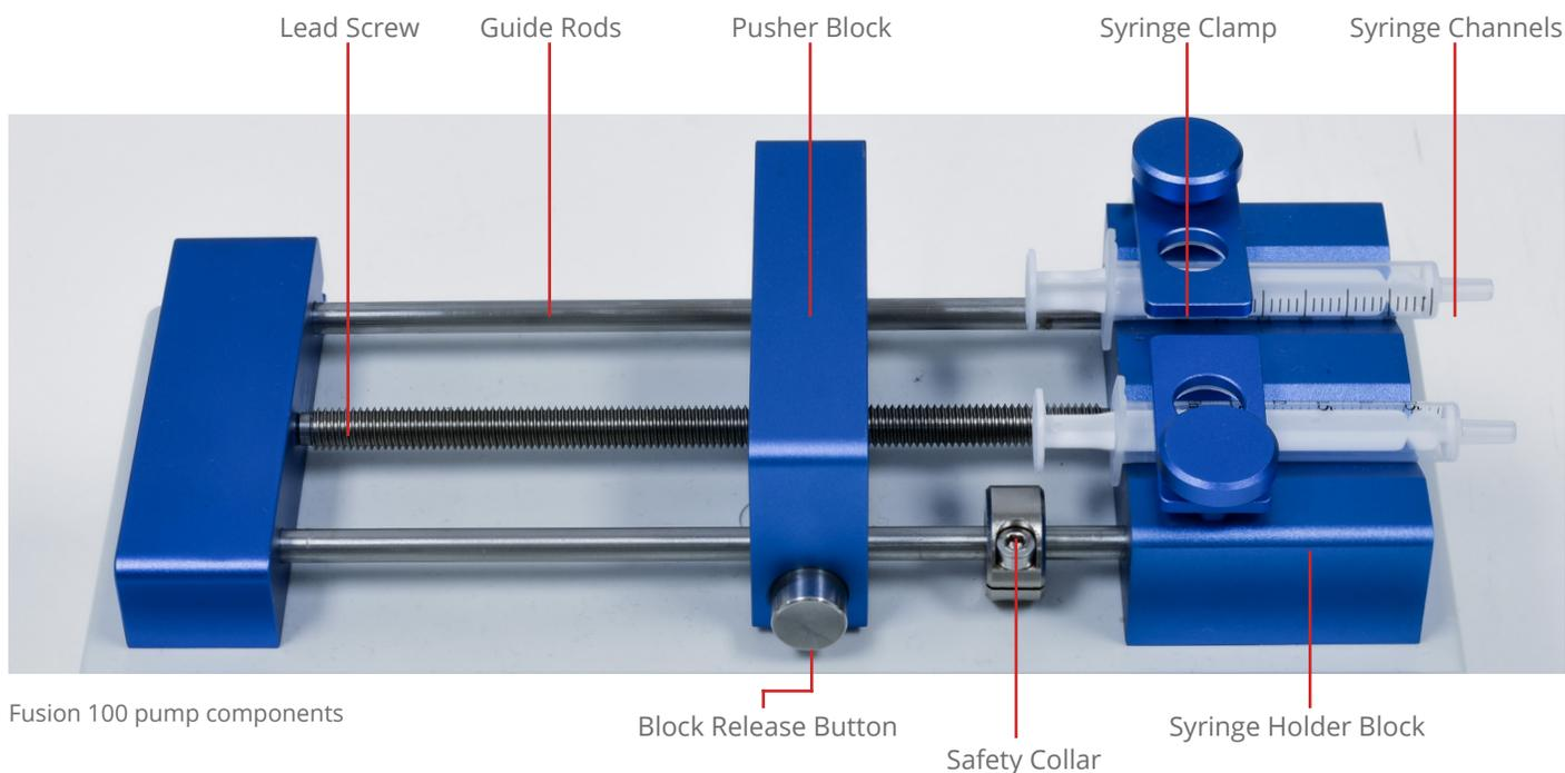
All Fusion Series pumps have a single lead screw through which the pusher block is threaded. The pusher block moves when the lead screw turns. The two guide rods keep the pusher block horizontal and perfectly perpendicular to the lead screw. The block-release button disengages the pusher block from the lead screw, which allows the pusher block to be easily moved to a new position as long as the button is held. Releasing the button will lock the pusher block back in place.
