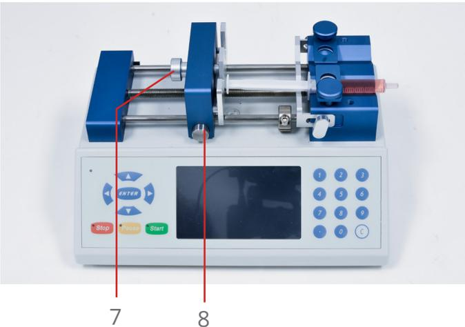
1. If necessary, move and tighten the infusion safety collar (see Adjusting the Safety Collar).
