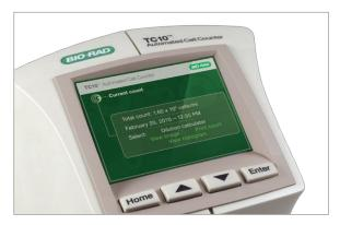
Fig. 3. Current count screen showing a total cell count (without trypan blue dye).
