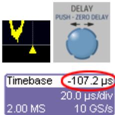
**Trigger Delay** - This indicator is located along the bottom edge of the grid. Trigger delay allows you to see the signal prior to the trigger time.
