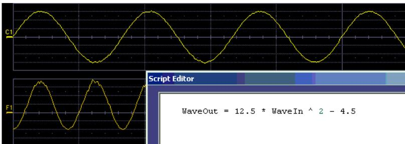
Example 3 below doesn't use the input data at all. The middle waveform (F2) is a "golden waveform", in this case a perfect sine (subject to 16-bit resolution), that was created using a VBScript. The lower trace (F3) is a subtraction of the acquired waveform (upper trace) and the golden waveform. The subtraction (of course) contains all the noise, but it also shows the presence of a very small square wave signal.
