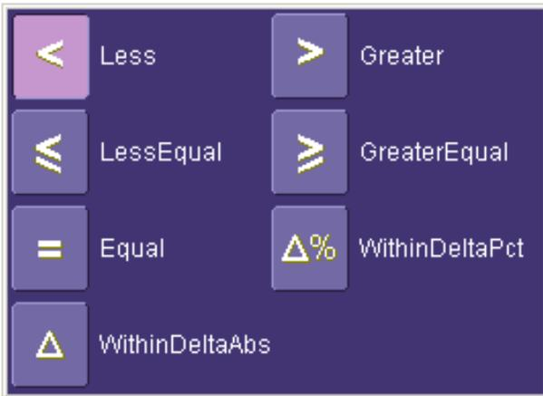
At the touch of a button, test results can also be compared to these standard statistical limits:
