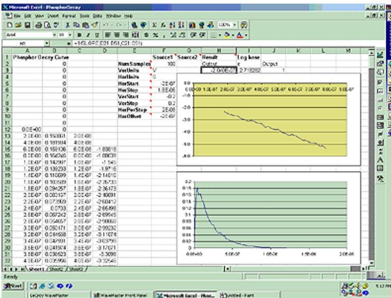
Here we see the input data in column B (with a time scale in A) created using the contents of cell F9, Horizontal Per Step. The logarithmic data are in column D, with the time scale repeated in C. The output appears in cell H3, using the formula **=1/SLOPE(D21:D51,C21:C51)**.
