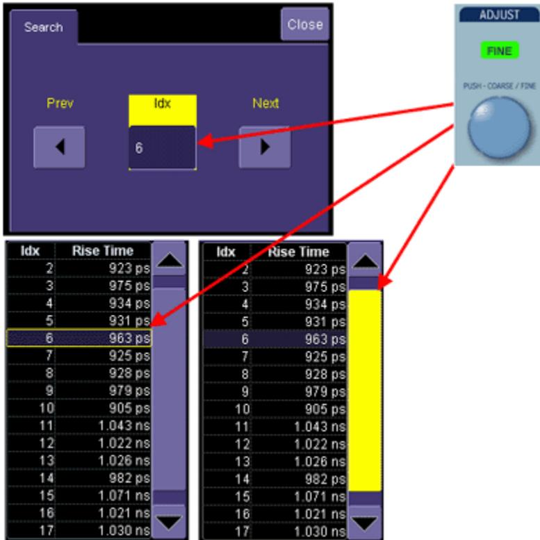
When the table contents are too numerous to fit in a single table display, a scroll bar will appear. By touching the scroll bar to highlight it, you can use the Adjust knob to quickly scroll through the table. In this case, however, the selection of edge will not change.
