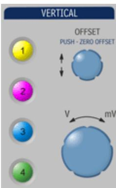
2. Turn the volts per division knob. Or you can touch inside the **Volts/Div** field and type in a value using the pop-up keypad.
