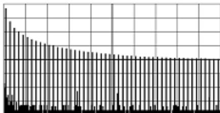
**In low-pass filtering:** The spectrum of a square signal before (left top) and after (left bottom) enhanced resolution processing. The result clearly illustrates how the filter rejects high-frequency components from the signal. The higher the bit enhancement, the lower the resulting bandwidth.
