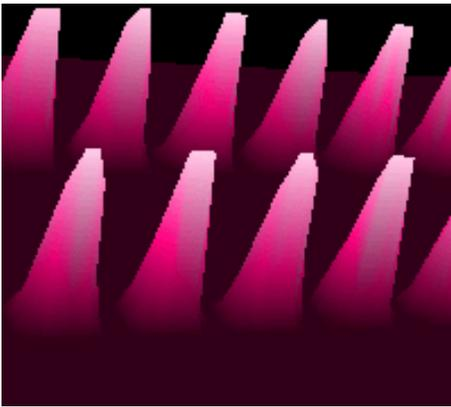
Here is a **monochrome** (analog) view of the same waveform. The lightest areas indicate highest intensity, corresponding to the red areas in the solid view.
