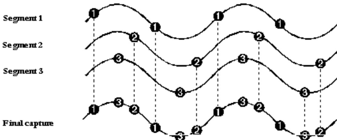
**Note:** RIS mode is not available when the oscilloscope is operating in Fixed Sample Rate mode.
