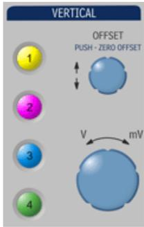
Turn the vertical offset adjust knob directly above the channel button whose waveform you want to move vertically. Or you can touch inside the **Offset** field and type in a value on the pop-up keypad. To set the vertical offset to zero, press the vertical offset adjust knob for the channel you want to adjust:
