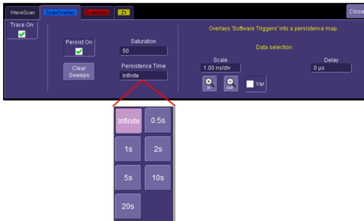
In the acquisition shown below, we have scanned for rise times greater than 1.4 ns. WaveScan has located six edges that meet this criteria, one of which is greater than 2 ns. This slowest edge, which appears in the persistence display, has been selected for zooming from the table. Note that it is also highlighted in the source view (top grid).
