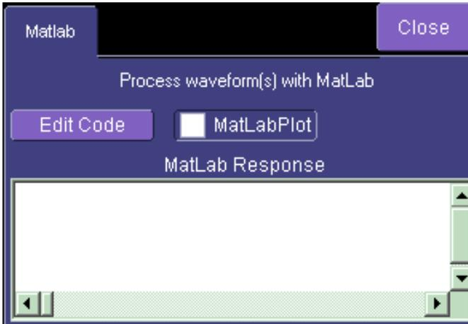
You can touch the **MATLAB Plot** checkbox if you want to see a plot in MATLAB as well as getting a result in the instrument.
