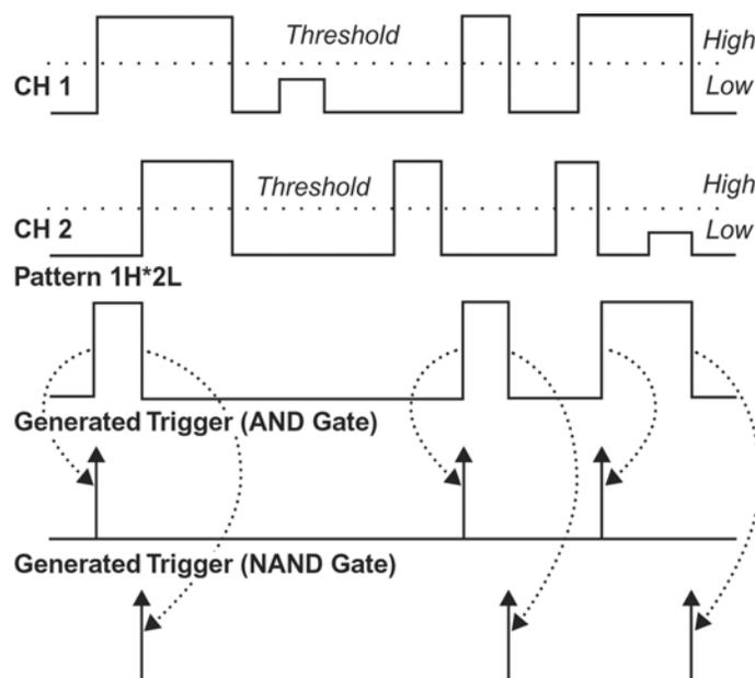
*Logic Trigger can be used in digital design for the testing of complex logic inputs or data transmission buses.*
