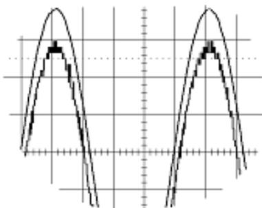
**To increase vertical resolution:** In the example at left, the lower ("inner") trace has been significantly enhanced by a three-bit enhanced resolution function.
