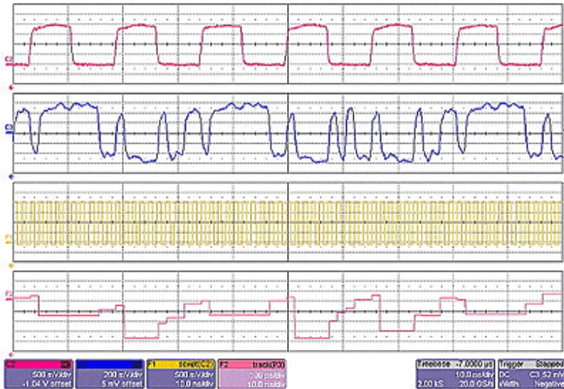
Example 4 is a measurement of DVI (Digital Video Interface) Data-Clock skew jitter measurement, using a VBScript to emulate the PLL.
