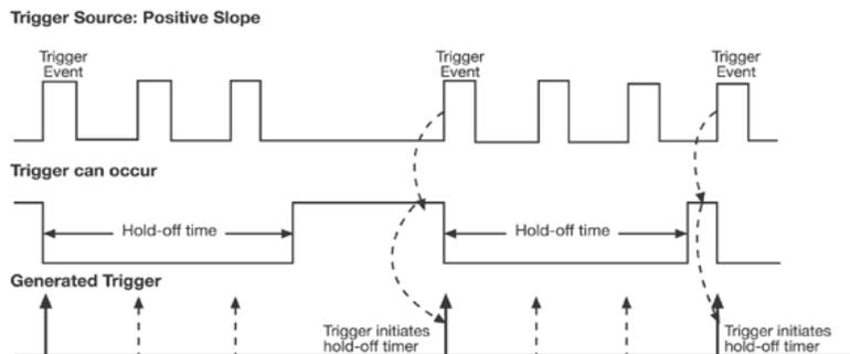
**Edge Trigger with Holdoff by Time. The bold edges on the trigger source indicate that a positive slope has been selected. The broken upward-pointing arrows indicate potential triggers, which would occur if other conditions are met. The bold arrows indicate where the triggers actually occur when the holdoff time has been exceeded.**
