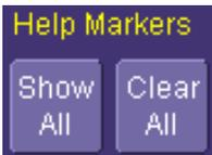
2. To turn off Help Markers for individual parameters, touch the **Px** tab for the parameter in question. Then uncheck the **Always On** checkbox. When you close this dialog, the Help Markers for this parameter will no longer be displayed.
