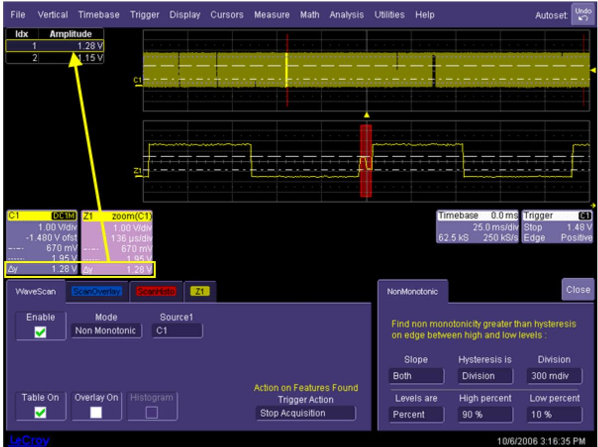
The hysteresis value is used to eliminate noise. A non-monotonicity is detected only when its amplitude is greater than the hysteresis. Therefore, when setting a hysteresis level, set a value that is greater than the amplitude of the noise.
