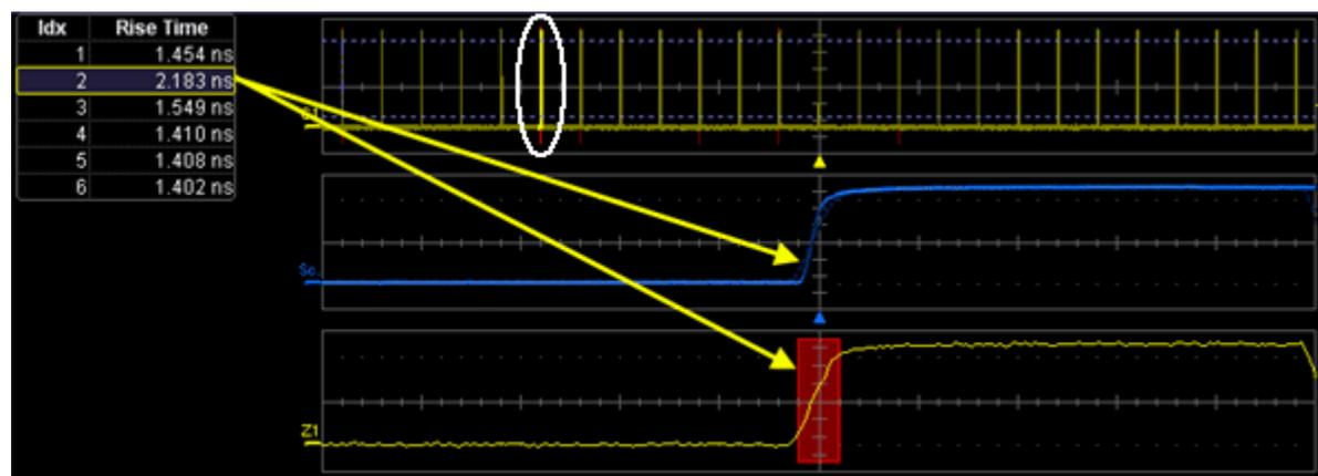
The horizontal scale of the overlaid traces can be expanded independently of the zoom trace. Here it is in the same scale as the zoom trace (5 ns/div), however.
