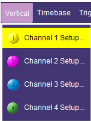
1. Touch **Vertical** in the menu bar, then **Channel 1**, for example, in the drop-down menu.
