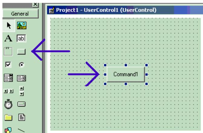
Create code for the buttons. A. Double click on the **Single** button. B. In the resulting code window, insert code to make the following subroutine:
