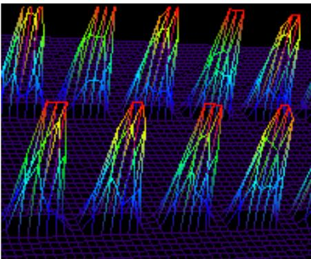
Here is a **wire frame** view of the same waveform in which lines of equal intensity are used to construct the persistence map.
