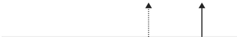
*Interval Trigger that triggers when the interval falls within the selected range:  $t_1$  = range's lower time limit;  $t_2$  = range's upper limit. The broken upward-pointing arrow indicates a potential trigger, while the bold one indicates where the actual trigger occurs on the positive edge within the selected range.*
