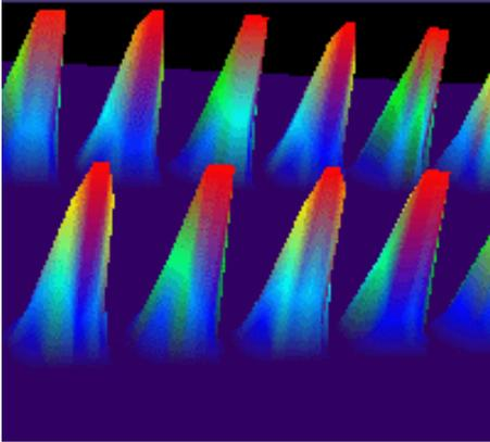
Here is an example of a 3-dimensional view of a square wave using the **solid** view of color-graded persistence. Saturation is set at 50%, with red areas indicating highest intensity. The X-axis has been rotated 60%; the Y-axis has been rotated 15%.
