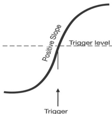
*Edge trigger works on the selected edge at the chosen level. The slope (positive or negative) is specified in the Trigger label permanently displayed below-right of the grid.*
