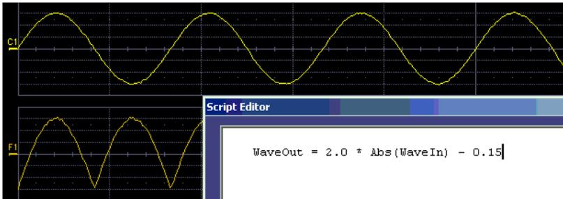
WaveOut is the waveform being returned to the instrument (F1 in this case). WaveIn is the input waveform (C1 in this case) You can see that the F1 result is displayed on the oscilloscope, and can be processed further.
