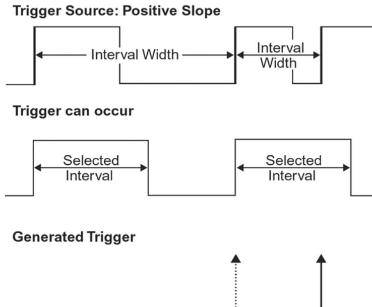
*Interval Trigger that triggers when the interval width is smaller than the selected interval. The broken, upward-pointing arrow indicates a potential trigger, while the bold one shows where the actual trigger occurs on the positive edge within the selected interval.*
