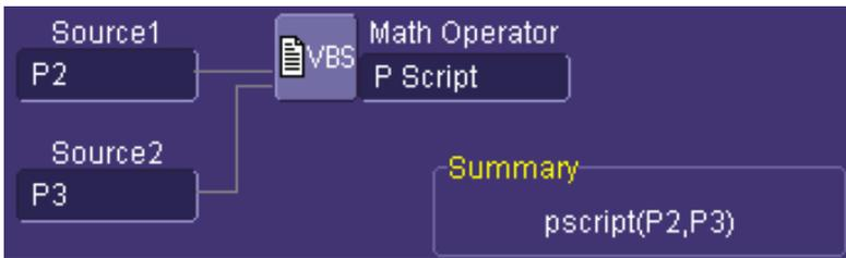
In addition to the arithmetic operations, the Parameter Math feature allows you to use VBScript or JavaScript to write your own script for one or two measurements and produce a result that suits your needs. Code entry is done in the Script Editor window directly on the instrument. You can also import an existing script.
