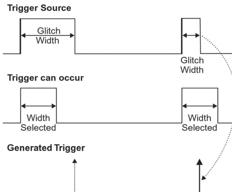
**Glitch Trigger:** In this example triggering on a pulse width less than or equal to the width selected. The broken upward-pointing arrow indicates a potential trigger, while the bold one shows where the actual trigger occurs.
