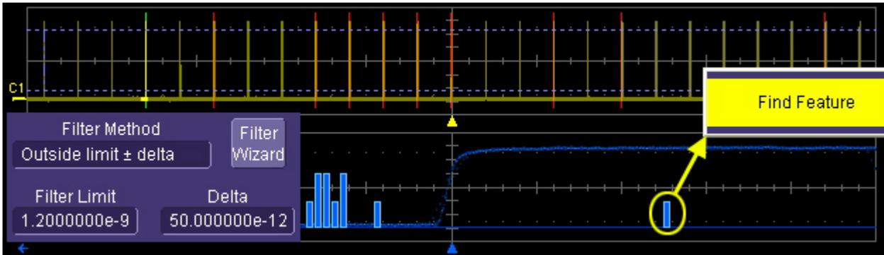
After Find Feature is confirmed, only the single bin of the histogram remains and information about the contents of the bin is displayed in the Filter Method area:
