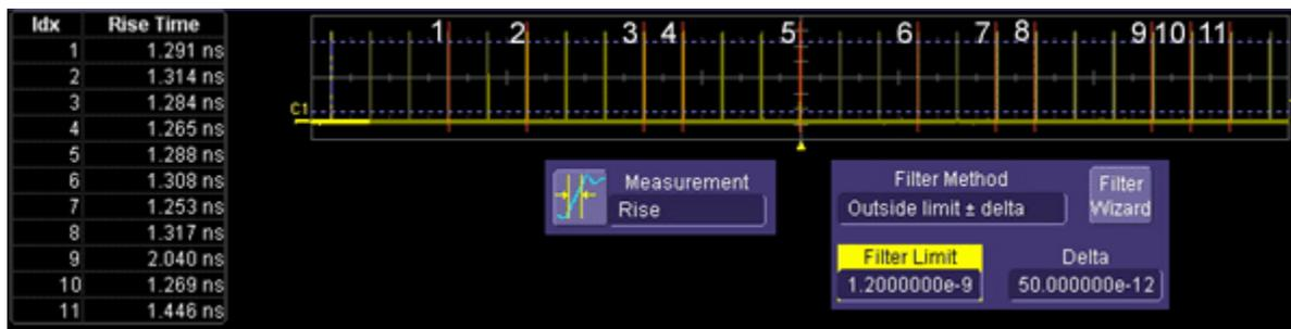
In this acquisition, WaveScan has located eleven edges that fit the search criteria (filter) of greater than 1.2 ns with a delta of 50 ps. Each of the found edges is highlighted with a red rectangle, and indexed to a table entry at left. Rise time values are also included in the table.
