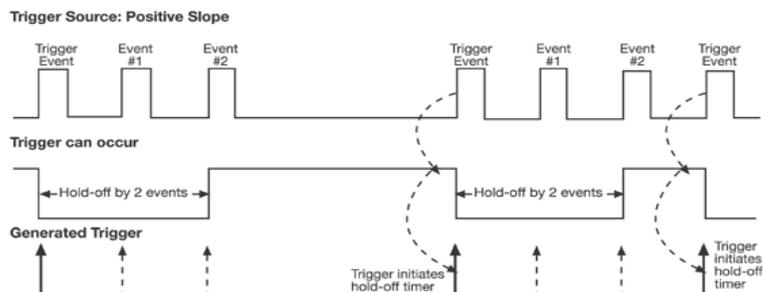
**Edge Trigger with Holdoff by Events (in this example, two events).** The bold edges on the trigger source indicate that a positive slope has been selected. The broken, upward-pointing arrows indicate potential triggers, while the bold ones show where triggers actually occur after the holdoff expires.
