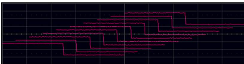
The number of segments you choose to display (80 maximum) can be less than the total number of segments in the waveform. For example, in the pop-up images above, the number of display segments is 10, but the total number of segments entered in the timebase dialog's **Num Segments** field is 100.
