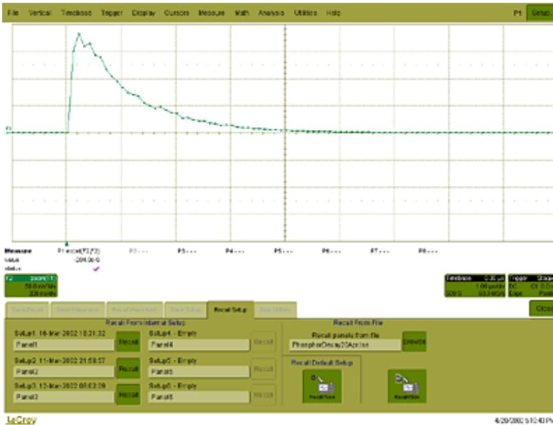
The pulse was generated by a formula of the form  $e^{-(t/TC1)} * e^{-t/TC2}$ , where TC1 and TC2 are time constants, The requirement is to measure the time constant TC2, using the portion of the trace where TC1 has negligible effect. This was done using Function F1, which is not a part of the measurement process.
