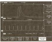
Dual window zoom is effective for managing the 500 K acquisition memory. FastFrame™ allows you to capture multiple events in a single record.
