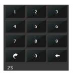
When the Goto Preset button is selected, the keypad changes to a numeric keypad. As digits are selected, they are displayed below the keypad. To cause the camera to go to the entered preset, select the Goto Preset button again.
