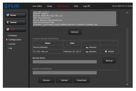
In the Custom Backup & Recovery section, click the Restore link associated with the factory.defaults configuration to restore the camera to its factory settings. This file can not be modified or deleted, so it is always available.
