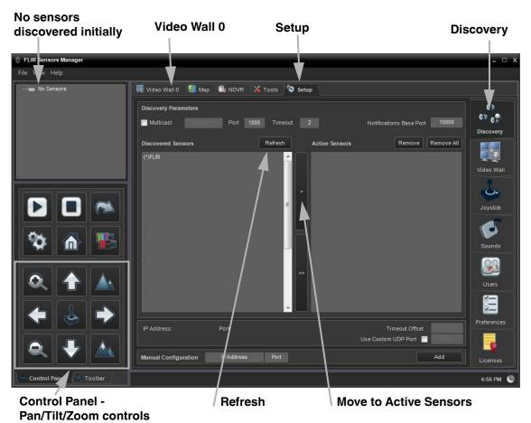
Click on **Setup**, if required, then the **Discovery** button on the side panel to bring up the Discovery Panel. The FSM software can automatically discover FLIR cameras on the network.
