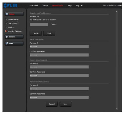
Note, as an additional security measure, it is possible to limit which computers have access to the web browser interface. At the top of the page under "Restrict Web Configuration", add a computer's IP address and click "Add". After all the allowed IP addresses are entered, select the Save button to save the changes. Note, once one or more addresses has been added to this list, **only** these computers will be able to log in to the web interface. Be sure to remember which addresses are allowed.
