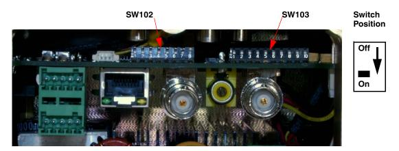
Figure 1-4: PT-Series Camera Configuration
