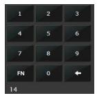
When the Function button is selected, the keypad changes to a numeric keypad. As digits are selected, they are displayed below the keypad. To execute the function, select the FN Function button again.
