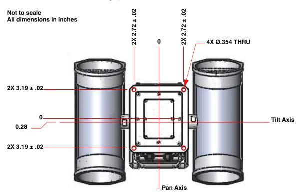
Figure 1-2: PT-Series Camera Mounting
