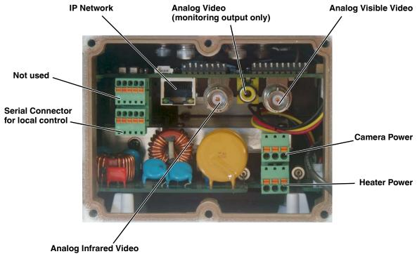
Figure 1-3: PT-Series Camera Connections
