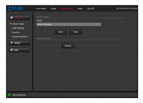
The basic camera configuration steps are accessed through the **Maintenance** menu, using the **Server** submenu on the left side of the page. The **LAN Settings**, **Services**, and **Security Options** selections are described below. Generally with these settings it is necessary to save the changes to make them effective, but it is not necessary to stop and restart the server.
