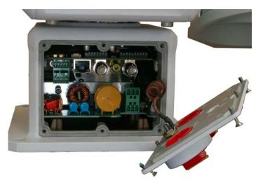
connecting them (the connectors will not fit through the cable gland). Leave the gland nuts loosened until all cable installation has been completed. Inspect and install gland fittings in the back cover with suitable leak sealant and tighten to ensure water tight fittings. Teflon tape or pipe sealant (i.e. DuPont RectorSeal  $T^{TM}$ ) are suitable for this purpose.
