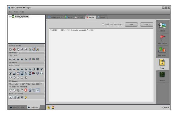
**Unable to View Video Stream:** If the video stream from the camera is not displayed in FSM, it could be that the packets are blocked by the firewall, or there could be a conflict with video codecs that are installed for other video programs.
