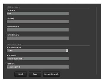
When the LAN settings are changed and the Save button is clicked, a pop-up message will appear to indicate the network interface should be restarted. Once all the changes have been made and saved, click on the **Restart Network** button at the bottom of the page.
