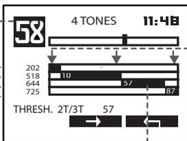
7 Adjust the sound frequencies and thresholds with
