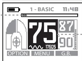
Discrimination enables undesirable targets to be rejected by raising or lowering a threshold below which certain metals are differentiated. The conductivity scale (0 to 99) for metal targets shown below will help you better understand the discrimination range and its limits, and see how it corresponds to the **digital display** of target conductivity on the remote control main menu.
