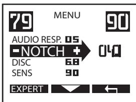
The Notch complements the discrimination: it enables a "target window" to be rejected whereas discrimination rejects all targets below a selected threshold. For example, if you detect a redundant, undesirable target in the ground, you can decide just to reject the corresponding conductivity group and continue to detect targets with a conductivity higher or lower than those in the group.
