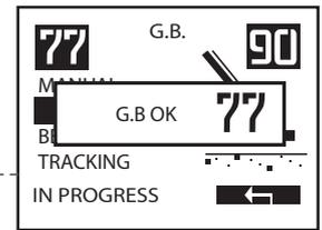
2 Press **START** and pump the coil on the ground several times until you obtain the display **G.B OK**
