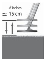
Press to grab the ground value while pumping the coil on the ground to calibrate and stabilise the DEUS. The number on the lower right of the screen shows you the new ground value.
