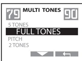
The FULL TONE mode will produce a slightly different tone for each target ID value based on a sliding scale. The higher the target's conductivity, the higher the tone will be. Iron typically will produce a low tone, while silver produces a high tone. See the figure on page 9 to see where specific types of targets fall in terms of conductivity.
