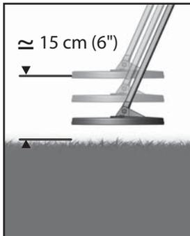
Pumping is a semi-automatic process which allows you to adjust the ground balance in a zone that you wish to search and have determined it as being an overall average soil type. Henceforth, the measured value of the ground is entered into the memory and used as the new active ground balance value.
