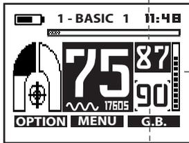
**The ground mineralisation index** (phase measured constantly for information).
