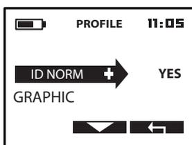
ID NORM (Standardization of the target ID) Allows the target value range to indicate the same for all the frequencies. Based on the 18Khz setting.
