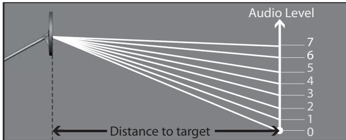
**Note :** By amplifying small signals you will also be amplifying small spurious false signals.
