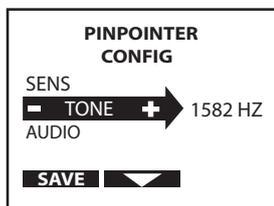
The MI-6 audio PULSE tone can be adjusted from the remote control, tones range from 120 to 1582 Hz. (Audio PULSE mode only)
