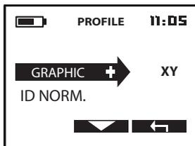
OSCILLOSCOPE DISPLAY XY: The target signature is displayed as an oscilloscope. The XY screen provides a visual assistance and may improve the identification of difficult targets. For example: The identification of targets that do not have a precise signature (some ferrous, cans ...). The XY profile can be selected as the default display. The display magnification of the XY trace has 10 levels of adjustment using the Zoom function.
