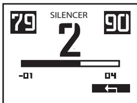
A few large iron objects or unusual shapes are often more difficult to discriminate. Often iron objects generate a few audible remnants of broken, or inconsistent signals (crackling). When you increase the silencer you are applying a filter which eliminates the crackling caused by ferrous. Level 2 represents a good compromise, but if you have difficulty identifying bottle caps, use level 4.
