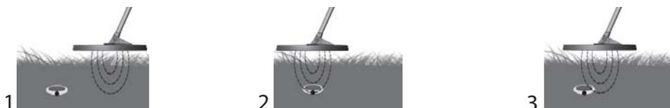
Position the coil barely off the ground (2 to 5 cm/ 1 to 2 inches) and to the side of the target. Press to calibrate the threshold.
