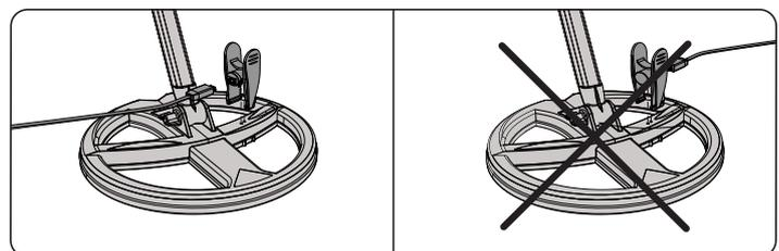
Ensure that the clamp is the right way round before connecting it to the coil. It can take up to 10 seconds for the led to activate.
