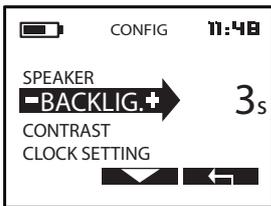
The remote control screen has a backlighting function which switch on as soon as any button is pressed and goes off automatically after a certain length of time. You can define this time in seconds:
