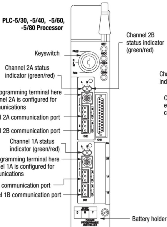
The PLC-5/30 processor has 2 communication ports and 1 serial port
