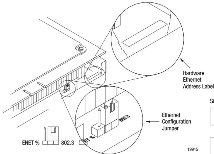
The Ethernet configuration jumper is located on the back of the processor. This jumper is factory set to 802.3, which is sufficient for most Ethernet networks. If your Ethernet network conforms to the DIX standard, set the jumper to ENET%.
