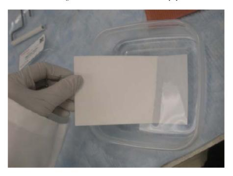
**13.** Place the presoaked iBlot<sup>™</sup> Filter Paper on the pre-run gel. Use the Blotting Roller to remove any air bubbles between the filter paper and gel.
