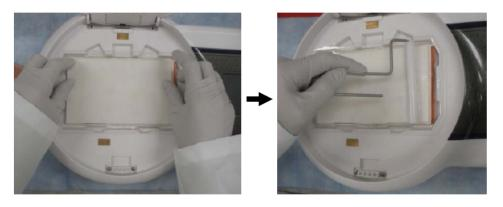
**14.** Remove and discard the white plastic separator from the Top stack.
