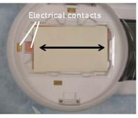
Orientation for iBlot™ 2 Mini Transfer Stack
