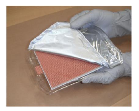
**3.** Separate the Top Stack and set it to one side of the bench with the transfer gel layer facing up. **Keep the Bottom Stack in the transparent plastic tray.**
