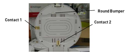
**2.** Hold the Lid with one hand, and remove the screw holding Contact 1. Discard both the screw and the contact.
