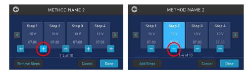
**4.** If a step is added, a screen appears to enter the desired voltage and time for that step. After the values are added, select **Done** to return to the Edit Method screen.
