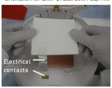
17. Use the Blotting Roller to flatten any protrusions in the transfer stack.
