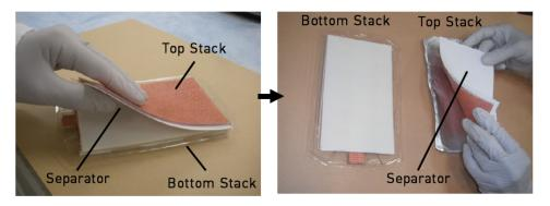
4. Place the Bottom Stack with the plastic tray directly on the blotting surface.
