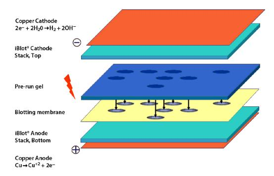
After the stack is assembled on the  $iBlot^{\mathbb{T}}$  2 Gel Transfer Device, and the appropriate Method is selected, the run is initiated. Complete transfer of proteins from the gel to the blotting membrane is accomplished in approximately 7–8 minutes. The rapid transfer without the need for external power supply or premade buffers is possible due to the following features of the  $iBlot^{\mathbb{T}}$  2 Dry Blotting System:
