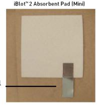
When properly assembled, the electrical contact of the iBlot<sup> $^{\text{TM}}$ </sup> 2 Absorbent Pad is aligned with the corresponding electrical contacts on the blotting surface of the iBlot<sup> $^{\text{TM}}$ </sup> 2 Gel Transfer Device to allow completion of the electrical circuit. See "iBlot <sup> $^{\text{TM}}$ </sup> 2 Transfer Stack specifications" on page 55 for dimensions of the iBlot  $^{\text{TM}}$  2 Absorbent Pad.
