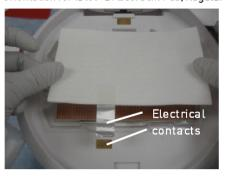
Orientation for iBlot™ 2 Absorbent Pad, Mini
