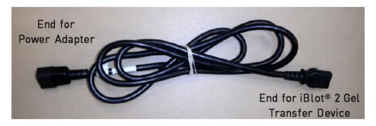
**IMPORTANT!** Be sure that the AC power switch is in the Off position ("Rear view" on page 9) before attaching the power cord. Attach the power cord to the AC inlet of the device first, and then to the electrical outlet. Use only properly grounded AC outlets and power cords.
