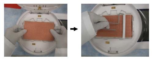
**16.** Place the iBlot<sup>™</sup> 2 Absorbent Pad on top of the iBlot<sup>™</sup> 2 Transfer Stack such that the electrical contacts are aligned with the corresponding electrical contacts on the blotting surface of the iBlot<sup>™</sup> 2 Gel Transfer Device.
