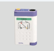
LX-5120/5160 Transmitter Dual-lead ECG, RESP
