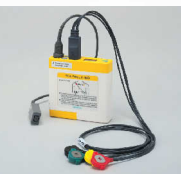
LX-5230/5630 Transmitter Dual-lead ECG, RESP, SpO 2
