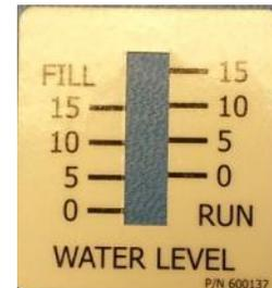
Once the tank is in place and the Acoustic Assembly is lowered into the bath, the water level should be read from the RUN side of the label.
