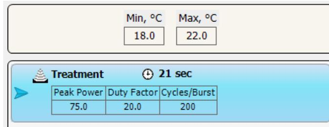
Average acoustic power (in Watts) and water bath temperature will be displayed numerically and graphically at the lower right corner of the Run Screen, along with a progress bar for the method being run:
