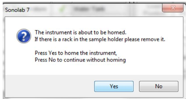
Click 'Yes'. The transducer and sample holder mechanical assemblies will move into position and the SonoLab 'Run' screen will display.
