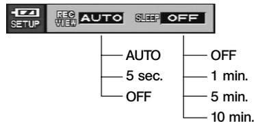
Ⓞ When item SLEEP is set to other option than "OFF", the LCD monitor turns off after the selected time period has elapsed while you perform no operation on the camera system.
