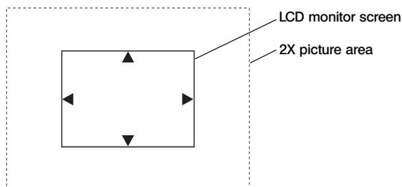
To view the hidden area of the picture, press and hold the EXPOSE button ③ while press one of the MOVE buttons ▲, ▼, ◀ and ▶ to move the picture in the desired direction.
