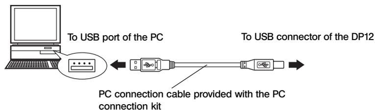
4. Connect the plug of the PC connection cable into the USB connector on the rear of the camera.
