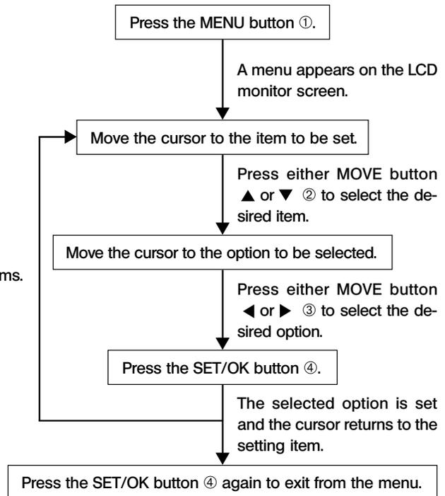
The setting is established and the menu disappears from the LCD monitor.
