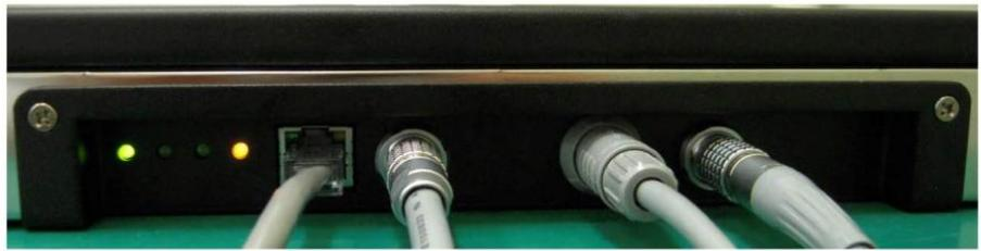
Figure 12: Detector cable connection
