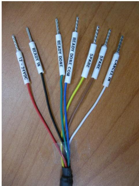
Figure 4:X-ray enable cable
