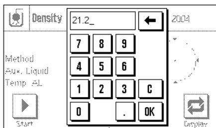
If you are using **water or ethanol as the auxiliary liquid**, enter its **temperature** using the **"Temp. AL"** function key. (Density tables for these two substances covering the temperature range from 10°C up to 30°C are stored in the balance; see also Sections 9.7 and 9.8.) The illustration here shows the corresponding input field (input in °C with 1 decimal figure).
