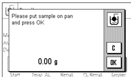
Press the **"Start"** function key to start the density determination. The balance will automatically carry out a taring, after which you will be prompted to put the solid body in place (weighing in air).
