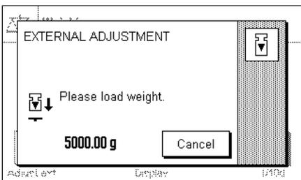
If there is a weight on the weighing pan at the time of the adjustment, the flashing display "0.00 g" prompts you to remove it. You will then be prompted to place the adjustment weight on the pan. The required adjustment weight is indicated at the lower edge of the window.
