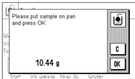
Press the "Start" function key to start the density determination. You will then be prompted to place the sample on the pan (without the gamma sphere).
