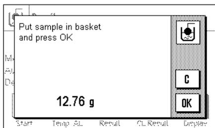
The result of the weighing is stored, after which you are prompted to immerse the solid body in the auxiliary liquid.
