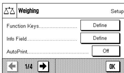
**Change application-specific settings:** If you want to change the settings for the active application, press the «≡» key. Information on the application-dependent settings can be found in the description of each individual application (Section 6ff).
