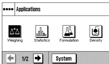
**Select the application:** If you do not want to work with the current application, use the «....» to select the application menu (or alternatively by touching the appropriate zone in the upper left-hand corner of the display). Touch the icon for the desired application, and the relevant software will load.
