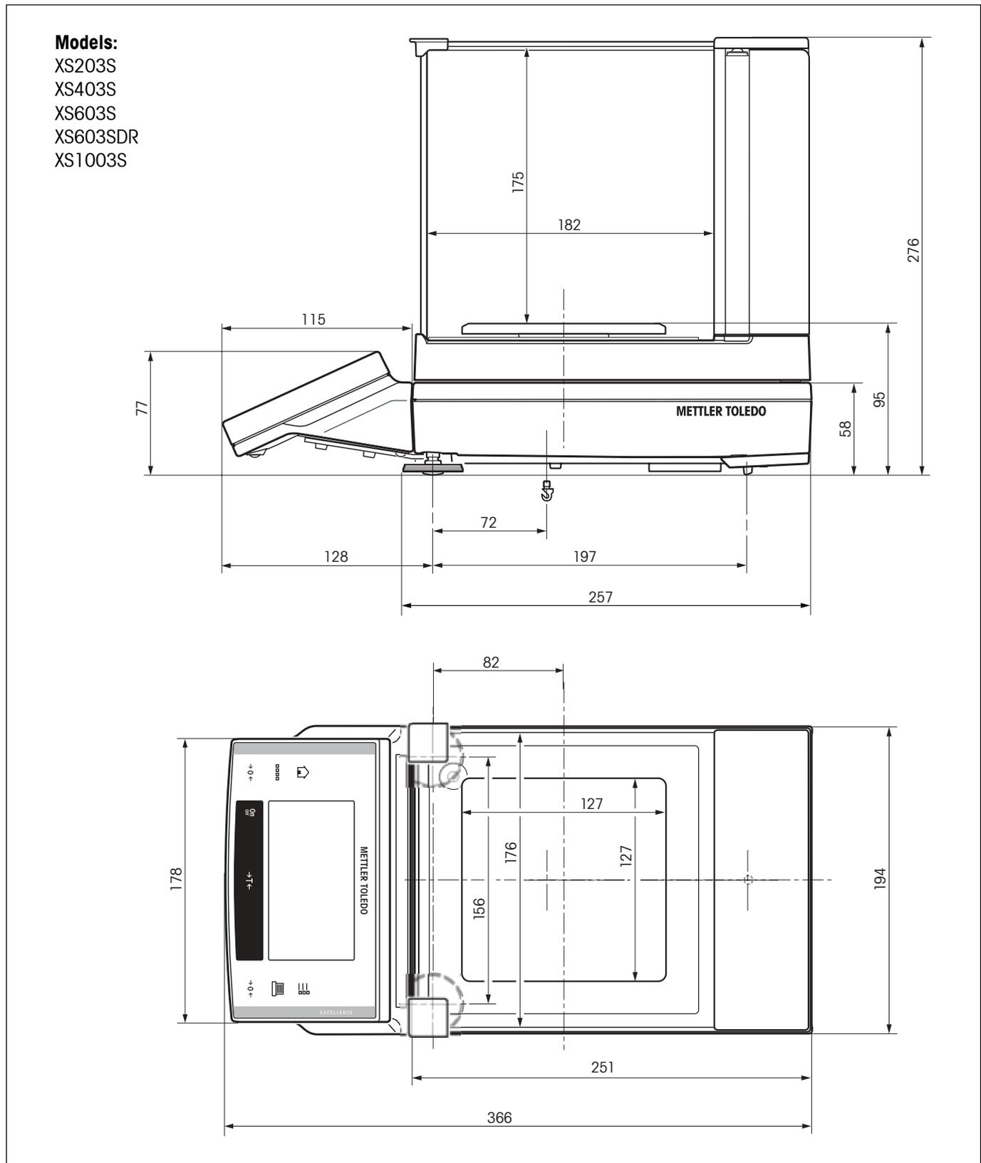
**16.3.2 XS precision balances with readability 10 mg, S platform with draft shield element**
