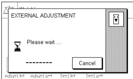
The adjustment process continues automatically once the required weight has been placed on the pan. The window shown here is displayed during the adjustment.
