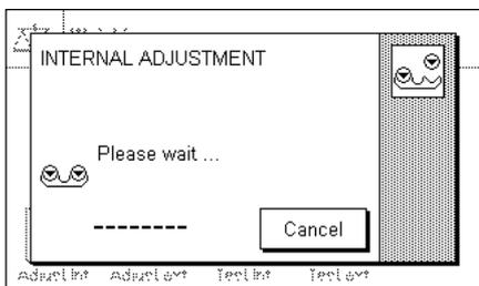
You can hear motors moving the internal weight into place and removing it again. The window shown here is displayed during the adjustment. The icons are animated, so that you can visually follow the adjustment process. You can halt the adjustment process at any time by pressing the "Cancel" key.
