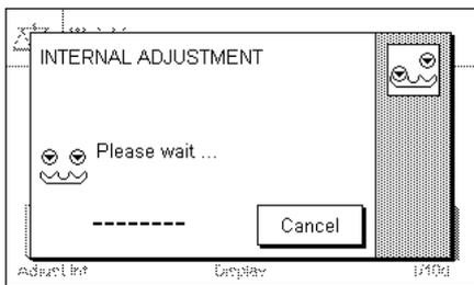
As soon as any load has been removed from the balance, and assuming that a key is not pressed for a period of 2 minutes, the adjustment automatically begins. A window appears in the course of the adjustment, informing you about the progress of the calibration. If you are working with the balance at the time of the adjustment, you can stop FACT with the "Cancel" button. The balance will carry out the adjustment at the next opportunity.
