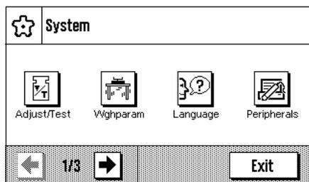
**Change system settings:** If you want to change system settings that apply to the entire weighing system, i.e. to all the applications, then press the «....» key and then the "System" button. The system settings are described in detail in Section 5.
