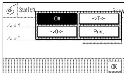
Select the desired function for each switch: "Print", zero setting («→0←») or taring («→T←»). If no switch is connected to the corresponding Aux connection, or if you want to deactivate it, select "Off".
