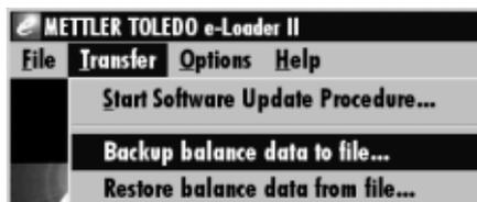
In order to save the current balance settings on a PC, start e-Loader II and call up the data backup function, as shown in the diagram here.
