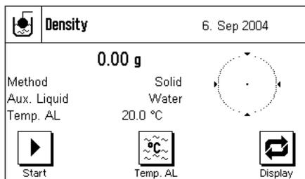
In the application-specific settings, select **"Solid"** as the method (Section 9.3.2) and specify the auxiliary liquid that will be used (Section 9.3.3).
