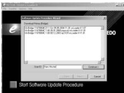
The balance now displays a list of the updates which have been performed. In this window you can enter a user identification "**User ID**" so that it is subsequently possible to trace who performed the software updating operation.
