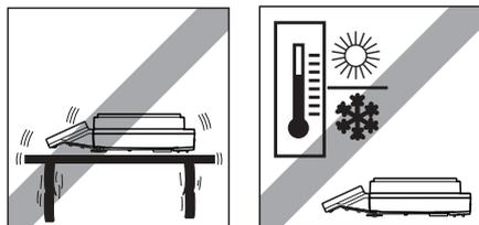
Select a stable, vibration-free position that is as horizontal as possible. The surface must be able to safely carry the weight of a fully loaded balance.
