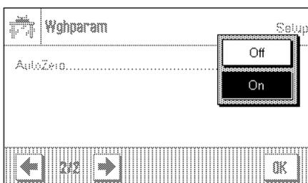
Automatic zero setting ("AutoZero") continuously corrects possible variations in the zero point that might be caused through small amounts of contamination on the weighing pan.
