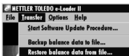
To copy the balance settings from the PC back into the balance, call the reload function, as illustrated here.
