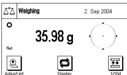
**Weighing:** Place the items to be weighed on the weighing pan, and close the glass draft shield (if present). As soon as the stability detector icon (the small circle to the left of the weight display) goes out, the display is stable and you can read off the weighing result. The stability detector icon is still visible in this diagram, and therefore the weighing result is not stable.
