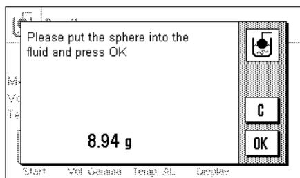
When the sample has been tared, you will be prompted to submerge the gamma sphere in the sample substance.
