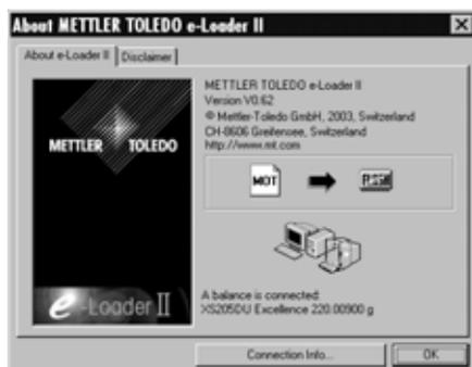
Before you update the software of your balance, please check in the "Help" menu that the communication with the balance is functioning. (In the example shown here, the e-Loader II is confirming that a balance is connected).
