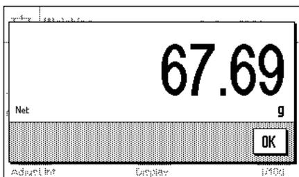
If you press the weighing result (**4a**) another window displays the weighing result in a larger size. This can be useful if you want to read the weighing result from some distance away. This window can be closed again by pressing the "OK" button on the screen.
