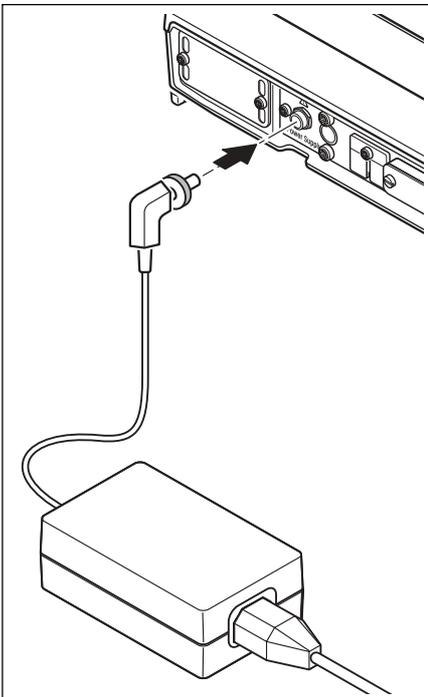
Your balance is supplied with an AC adapter and a country-specific power cable. The AC adapter is suitable for all line voltages in the range:
