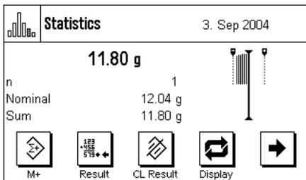
As soon as you have entered the target value and the tolerances the graphical filling guide ("SmartTrac") appears. This displays tolerance marks that make it easier for you to weigh up to the target value: You can add roughly the right amount of material until the lower tolerance value has been reached, and then, if necessary, make careful additions to reach the target value.
