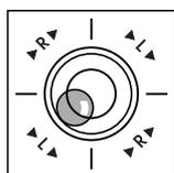
**Example:** The position of the air bubble illustrates which leveling screw you need to turn and in which direction so that the air bubble moves to the center.
