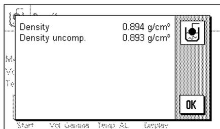
The balance now determines the density of the paste, and then displays the result (the compensated and/or uncompensated value, depending on the settings that you have made for output of the result, see Section 9.3.5).
