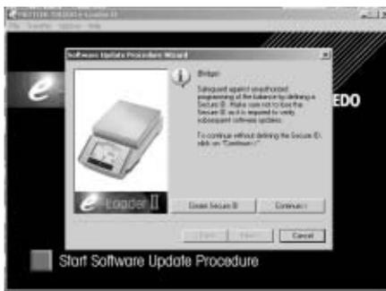
Before you start the actual updating operation, you have the possibility to define a **Secure ID** to protect the balance against unauthorized software updating operations. To do this, click on the "Create Secure-ID" button. If you do not wish to use this function, click on "Continue".
