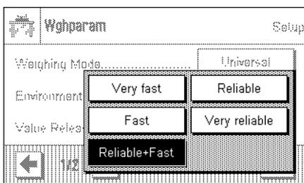
With this setting you can specify how rapidly the balance considers the measurement to be stable and therefore releases the value. The "Very fast" setting is recommended if you require rapid measurements whose repeatability is of lower significance. The "Very reliable" setting leads to measurements that are highly repeatable, but it lengthens the stabilization time. Three other intermediate settings can be selected.
