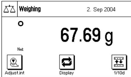
The factory setting of the balance displays the weighing result at a size so that it can easily be read. In this display mode neither the information fields nor the graphical "SmartTrac" filling guide are visible.
