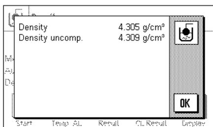
The balance now determines the density of the solid body, and then displays the result (the compensated and/or uncompensated value, depending on the settings that you have made for output of the result, see Section 9.3.5).
