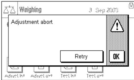
**An error occurred during the adjustment, and the process was aborted.** This message will also appear when you have cancelled the adjustment yourself. You can repeat the adjustment procedure, or can return to the application by pressing "OK".
