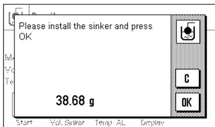
Press the "Start" function key to start the density determination. You are prompted to attach the sinker (weighing in air for taring).
