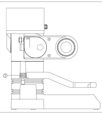
Figure 11: Immersion depth of the evaporation flask
