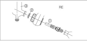
Figure 7: Sealing system RE
