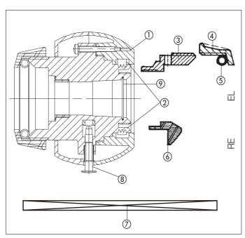
Figure 26: Cross section of bearing
