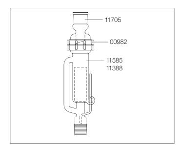
**"Soxhlet" extraction top**Using this accessory in conjunction with glass apparatus S you can carry our extractions.
