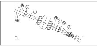
Figure 8: Sealing system EL
