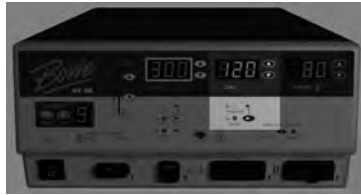
Figure 2 – 4 Controls for the Coag mode
