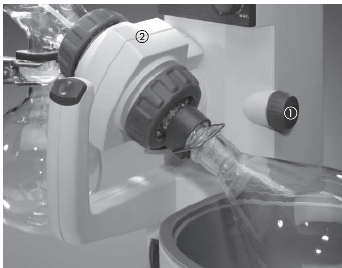
Picture 13: Drive unit with fixing screw
