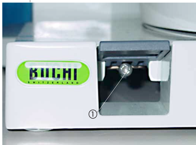
Picture 15: Adjusting tension of the servo jack rope
