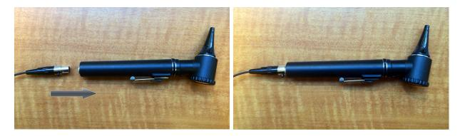
2) Connect the other end of the cable to the hole at the top of the Sensor Box, as shown below. Now the Sensor Box and the provided Instrumented Otoscope are connected.
