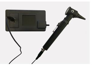
3) Connect the Sensor Box to the computer, using the USB Cable. When powered up, the Sensor Box will display a green graph with the motion of the otoscope. (You may have to restart the OtoSim 2<sup>™</sup> Sensor by
