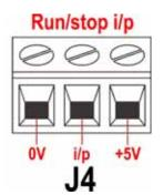
Remote run/stop: connect a remote switch between the  $\mathbf{i/p}$  terminal and the +5V terminal of the Run/stop i/p connector (J4). Alternatively a logic input may be applied to the  $\mathbf{i/p}$  terminal, ground to the  $\mathbf{0V}$  terminal. High input stops the pump, low input runs the pump. With no connection or with the switch open, the pump will default to running. To change or set the sense of the run/stop input, see 16.5 Remote stop in the Setup menu.
