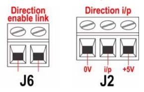
To enable remote direction control and disable the **DIRECTION** (SHIFT, 1) key on the keypad, link the terminals of the Direction enable link connector (J6). Important: Apply no voltage whatever to the Direction enable link. Connect a remote switch between the +5V terminal and the i/p terminal of the Direction i/p connector (J2). Open switch for clockwise rotation,
