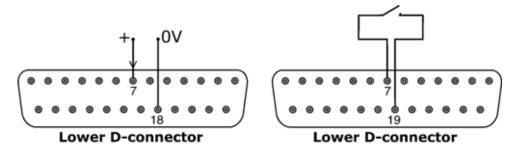
Remote run/stop: connect a remote switch between pins 7 and 19 of the lower D-connector. Alternatively a logic input may be applied to pin 7 of the lower D-connector, ground to pin 18. High input stops the pump, low input runs the pump. With no connection or with the switch open, the pump will default to running. To change or set the sense of the run/stop input, see 16.5 *Remote stop* in the Setup menu.
