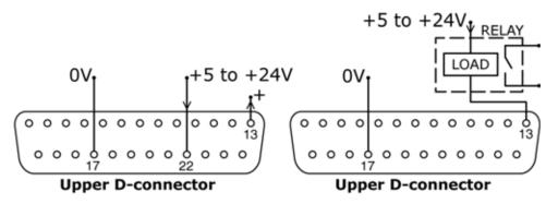
Output 3 is taken from pin 13 of the upper D-connector, depending on the logic state of the function assigned to Output 3. Alternatively, a load such as a relay coil may be connected to pin 13, ground to pin 17. Current will flow through the circuit depending on the logic sate of the function assigned to Output 3. Do not connect to any device requiring more than 50mA.
