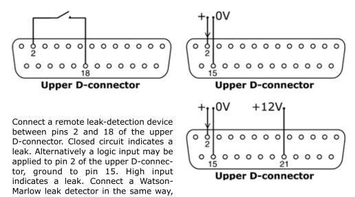
drawing 12V to power it from pin 21 of the upper D-connector.
