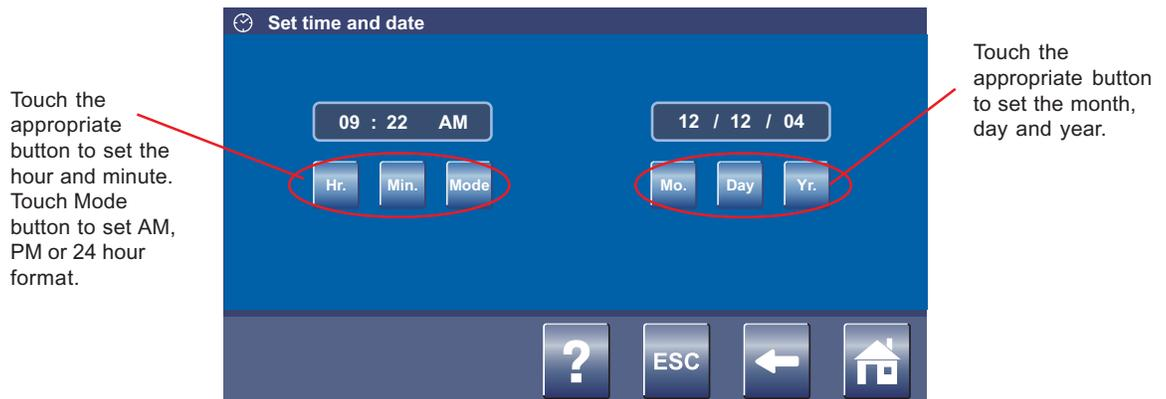
Figure 27. Set Console Time and Date Screen - Advance User Mode
