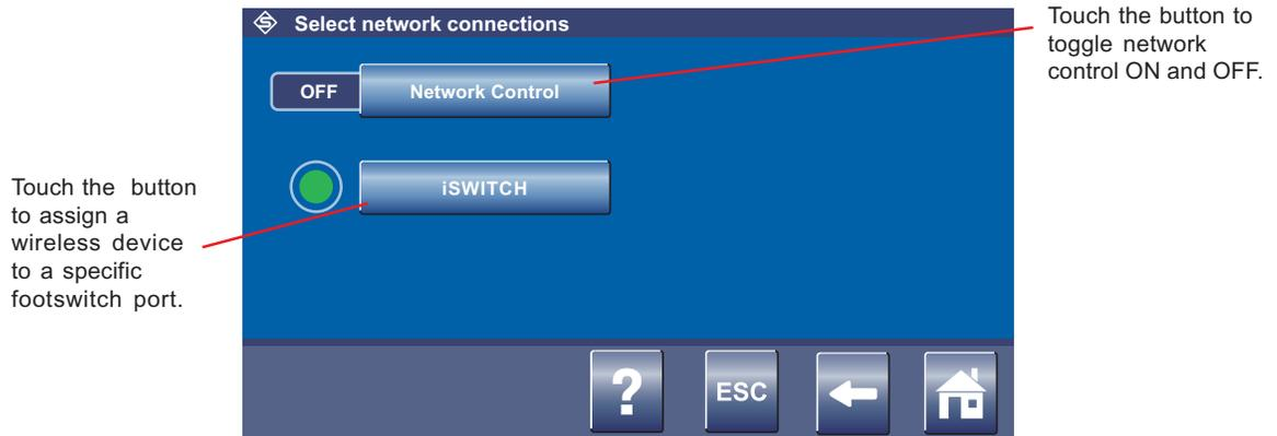
Figure 26. Select Network Connections Screen - Advance User Mode
