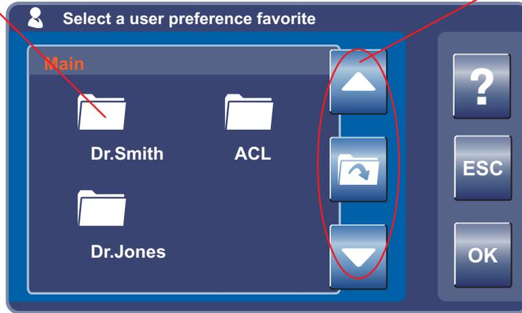
Touch arrow buttons to scroll through and view the available folders. Select a folder and touch the Open Folder button to access the files.
