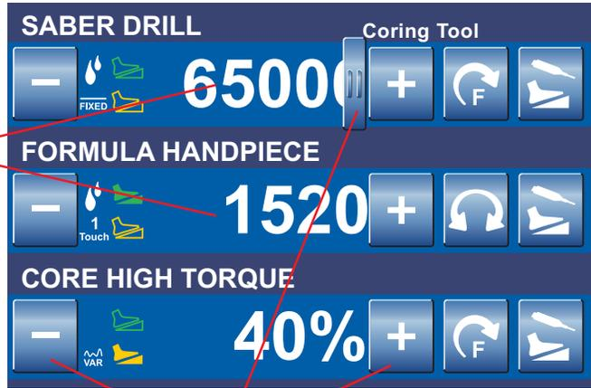
Touch the adjustment buttons (or slider bar that becomes visible when touching the speed value) to increase or decrease the speed (power) set point.
