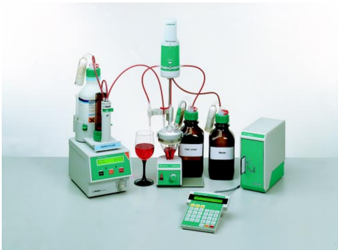
The 711 Liquino in the SMPL mode together with the 719 SET Titrino for automatic wine analysis
