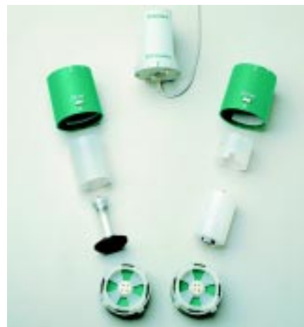
Detailed view of the Dosing Unit; left with glass cylinder, right with ETFE cylinder. Note the unique flat stopcock with its four bores
