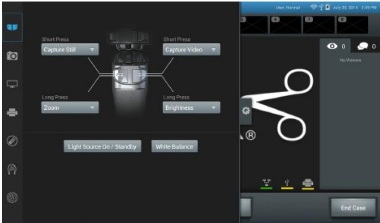
**Figure 29 -Camera Head Button Change During Case**
