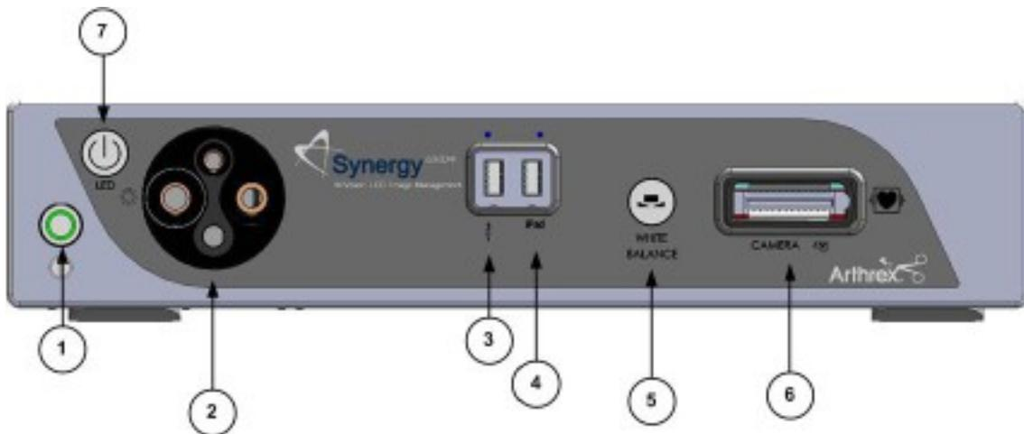
Figure 1- Synergy<sup>UHD4</sup> Front Panel [AR-3200-002X]
