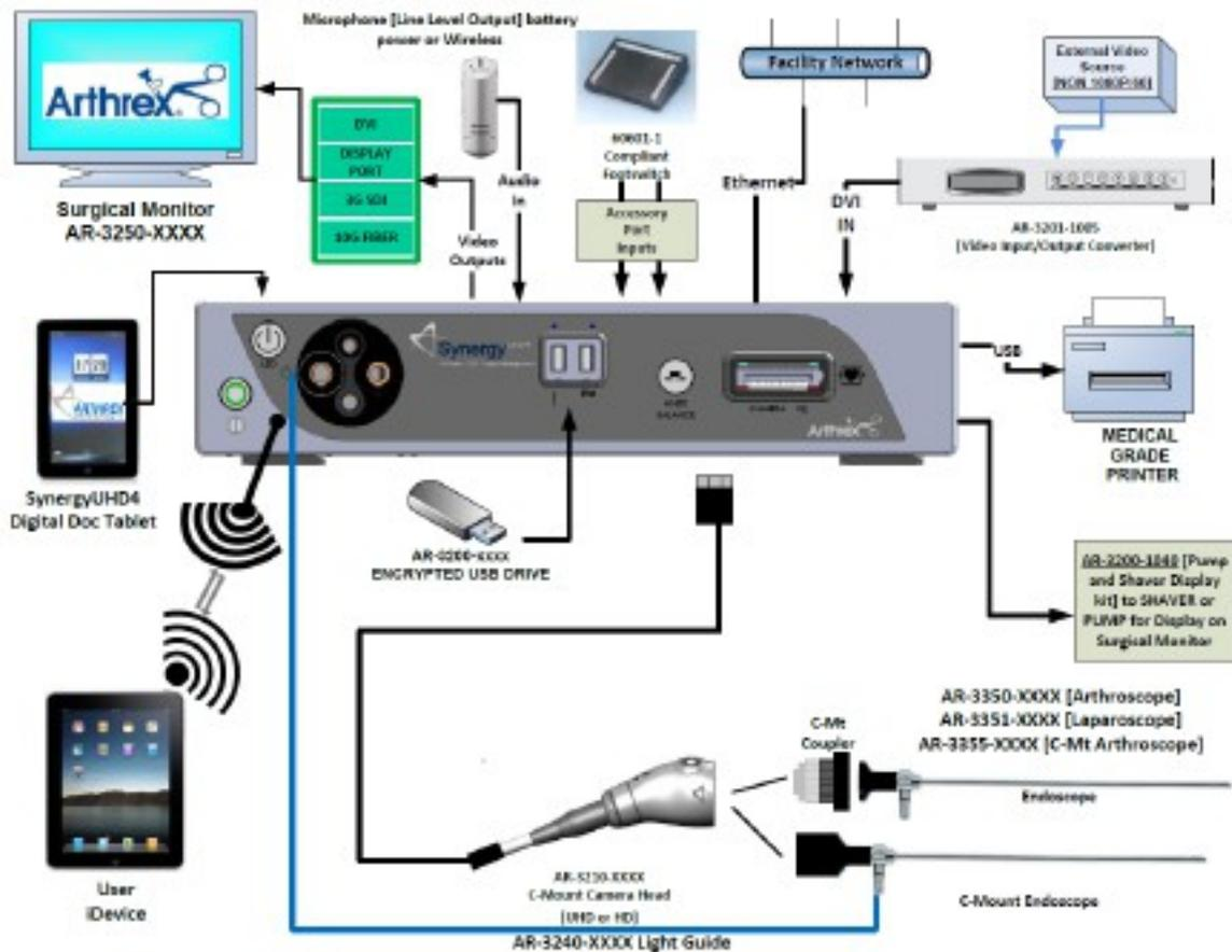
Figure 13- Synergy<sup>UHD4</sup> Typical Interconnect Diagram [C-MT Heads]
