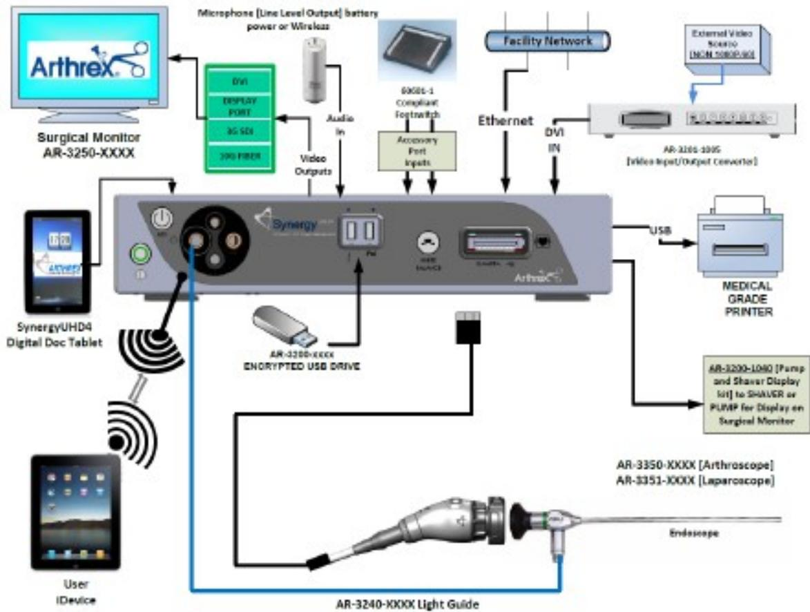
Figure 12- Synergy<sup>UHD4</sup> Typical Interconnect Diagram with OPTIONAL Digital Documentation Tablet [Integrated Optics Heads]
