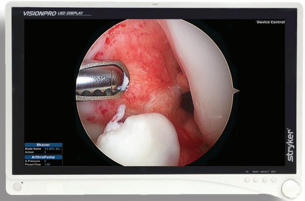
Critical Device status feature allows for customisable data to be displayed on the flat panel monitor, allowing for seamless reference of Arthroscopy Pump Pressure, Insufflator Pressure, Flow rates, Lightsource Brightness etc
